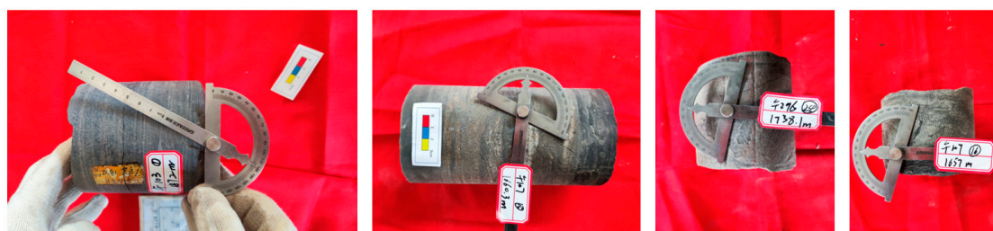
Figure 6. Locations of high-angle fractures in core samples.
