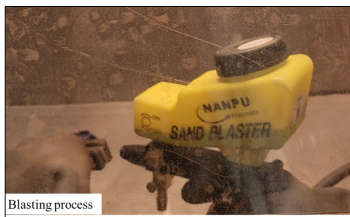
Figure 1. Steel shot blasting in an enclosure using a NANPU sandblaster gun connected to an 85 psi compressed-air supply.
