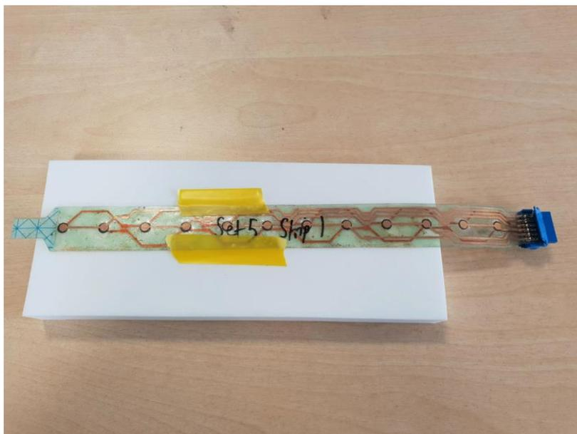
**Figure 1.** Image of one sensor strip attached to a 3D-printed block for examination of response under load, with 12 sensors and a connector head on the top to allow connection to the control board.
