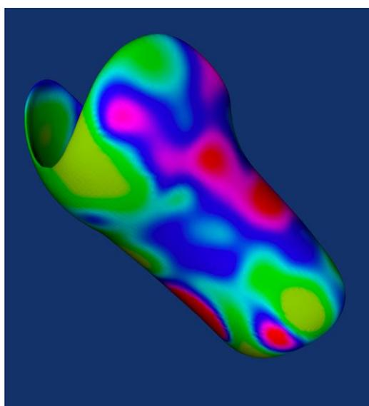
**Figure 3.** Radial basis function interpolation applied to a 3D computational model of a prosthetic socket using data.
