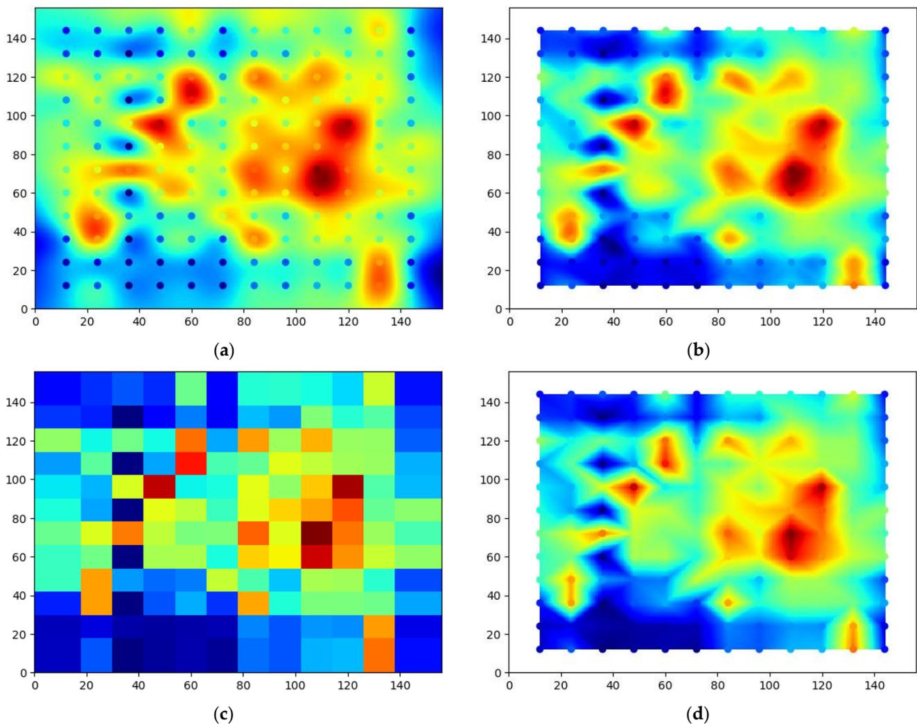
**Figure 2.** The 2D output of pressure sensor data with (a) radial basis function, (b) Clough–Tocher, (c) nearest-neighbour, and (d) Linear interpolation methods from a single time point.
