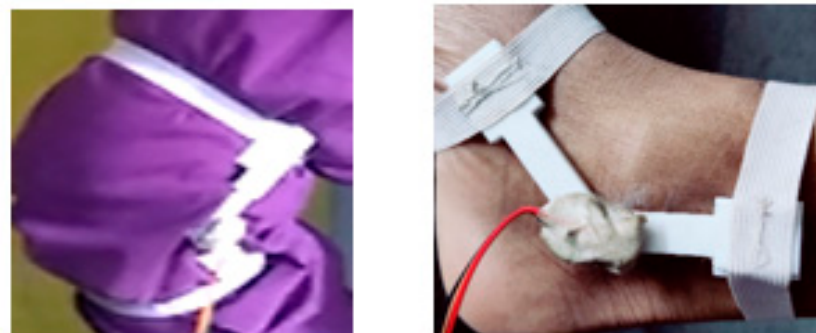
Figure 2. Pictorial Representation of Rotary Encoder connected at knee and ankle joints.
