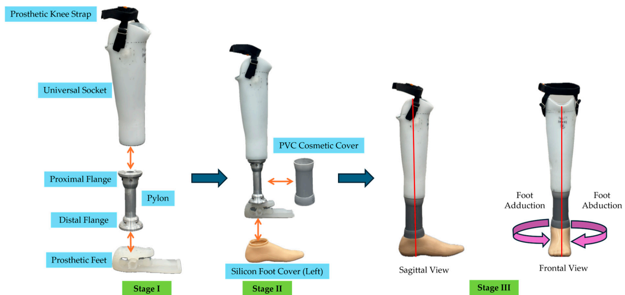
Figure 2. Assembly of the transtibial Mercer Universal Prostheses (MUP) with standard “Neutral” socket alignment. Stage I shows an assembly of the universal socket with the prosthetic foot via modular proximal and distal flange components; the pylon can be cut for prosthetic length adjustment. Stage II includes a Silicon foot cover (either Left or Right foot) and PVC cosmetic cover for the pylon and flanges to enhance the aesthetic of the prosthetic device and reduce water leaking inside of the prosthetic foot. Stage III shows the completed MUP device with the “neutral alignment” axis or mechanical axis indicated as a red line. The MUP only provides adjustments of foot adduction/abduction in the transverse plane.
