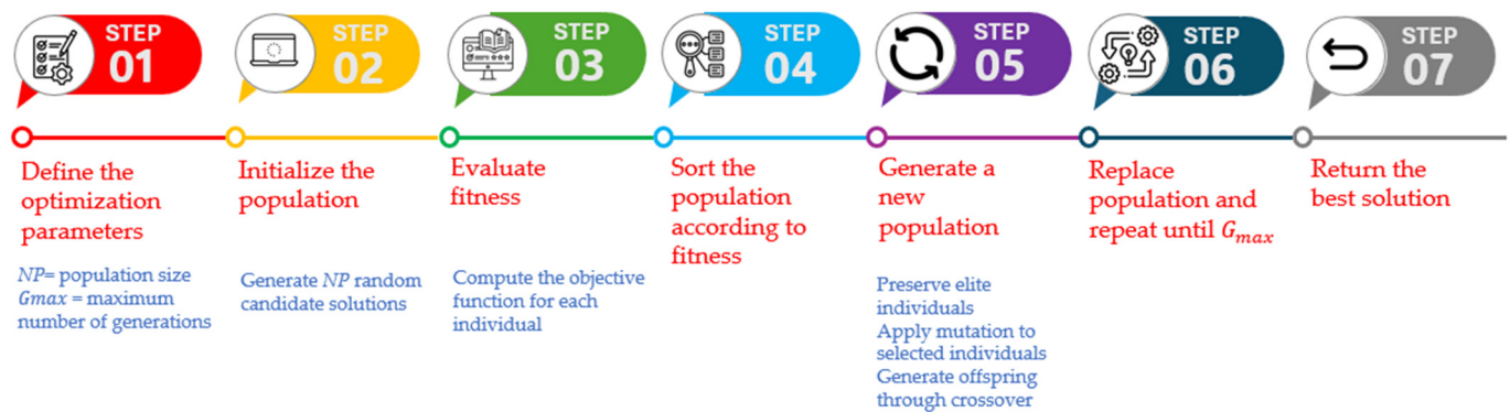
Figure 7. GA methodology to obtain the four-bar mechanism parameters.
