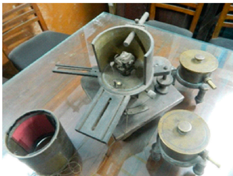
Figure 8. X-ray Diffraction Apparatus built by SN Bose. (Courtesy: Prof. Alok Mukherjee).
