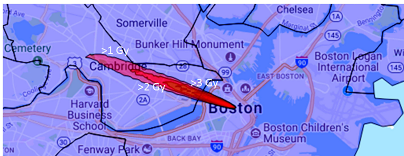
Figure 3. Capacity of ADCI-HT for dose estimation in a high yield mass casualty. HPAC-derived plume presented intersects with contours of >2 Gy include Boston, Suffolk County, Massachusetts (population = 673,184) and Cambridge, Middlesex County, Massachusetts (population = 110,651), leading to a total population of 783,835. Extrapolating from 6480 sample run (1.3 h for 4 nodes), the time required for ADCI-HT to analyze samples from the total population would be 157.25 h or 6.5 days.
