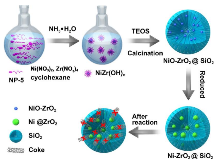
Figure 3. Illustration of the fabrication method of the Ni-ZrO 2 @SiO 2 catalyst with ultra-high coking and sintering resistance for the DRM reaction. Reproduced with permission from reference [89].
