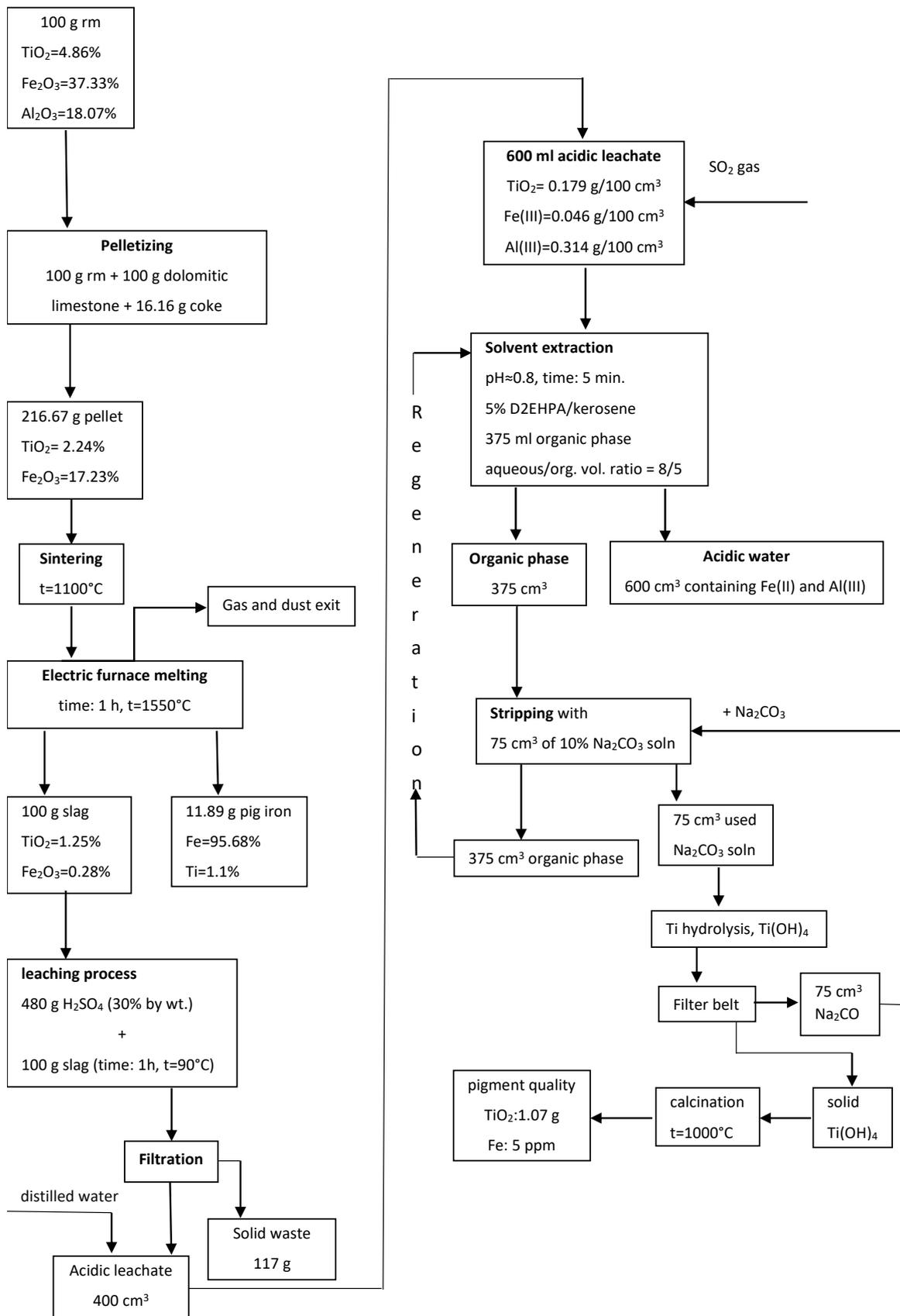
**Figure 3.** The schematic diagram of comprehensive processing of red mud via reduction roasting–smelting–sulfuric acid leaching–solvent extraction. Reproduced from [13].
