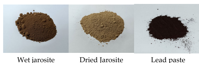
Figure 1. Metallurgical wastes used for the pyrometallurgical trials.
