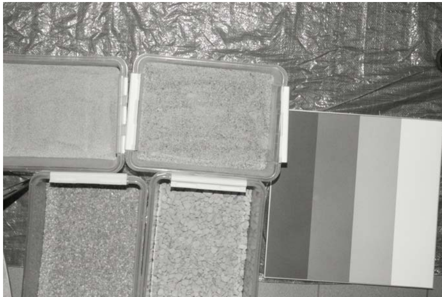
Figure 2. A Fuji camera NIR-image of the samples, taken from the scissor lift. The gravel samples are seen on the left and the 4-step Spectralon panel on the right side.
