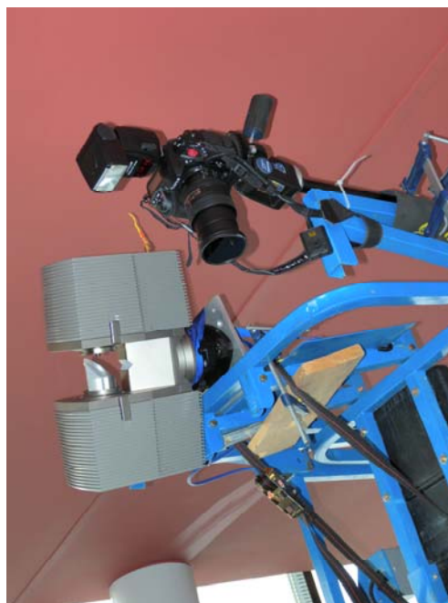
Figure 1. The FARO Photon scanner and Fuji IS PRO camera mounted on a scissor lift rack, facing downwards. The samples are placed below the lift.
