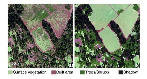
**Figure 2.** The first step of the OBIA process: the image segmentation process: (a) a fine spatial resolution color infrared image of an oak forest stand with dead trees; (b) the corresponding image segments.
