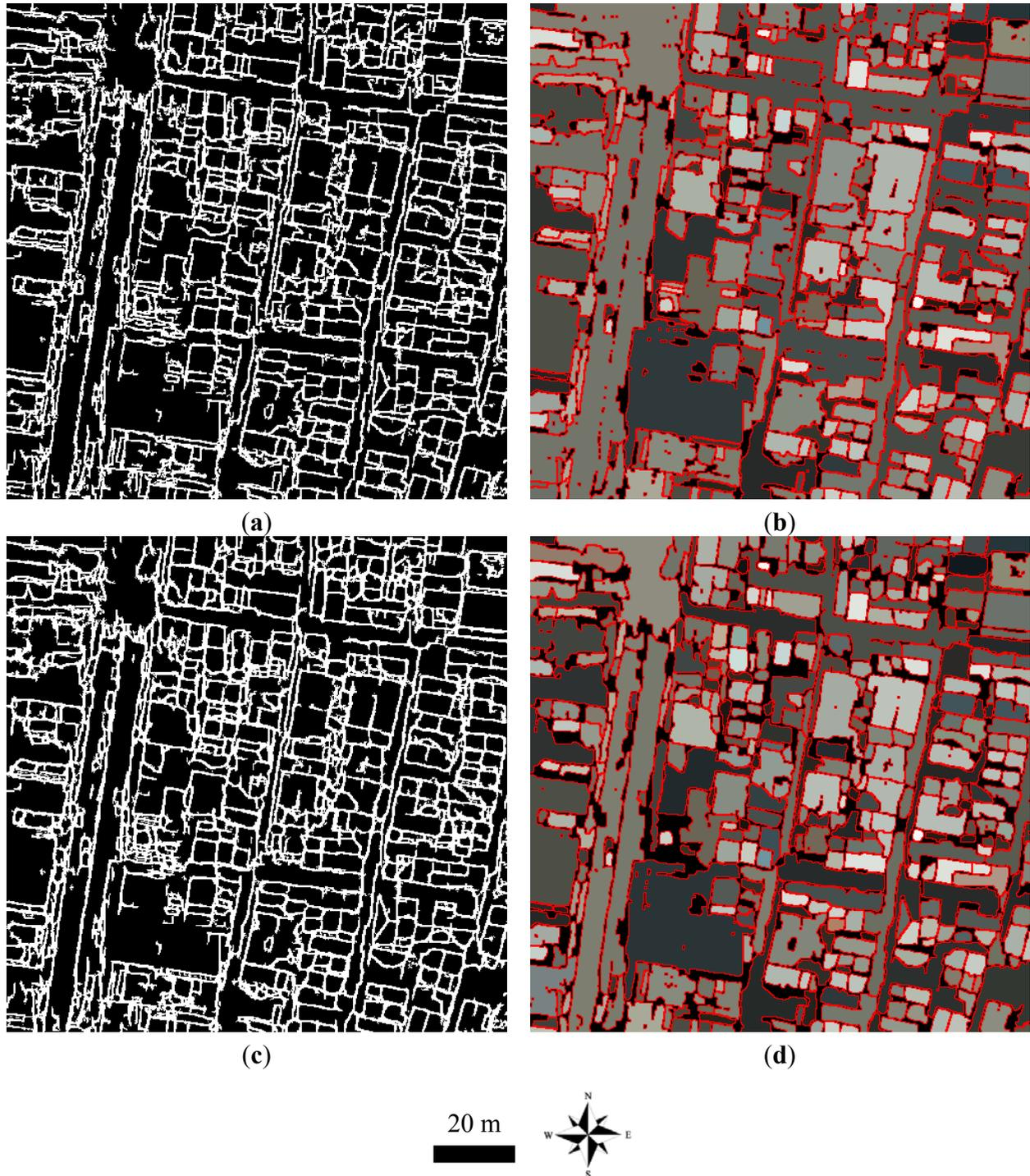
**Figure 15.** Edge completion by using combined edges: **(left)** extracted edges and **(right)** segmentation results using these edges. **(a)** Results with  $\Delta d_i = 40$ , **(b)** results with  $\Delta d_i = 30$ , **(c)** results with  $\Delta d_i = 20$ , and **(d)** combined edges when edges with  $\Delta d_i = 40, 30$ , and  $20$  were merged.
