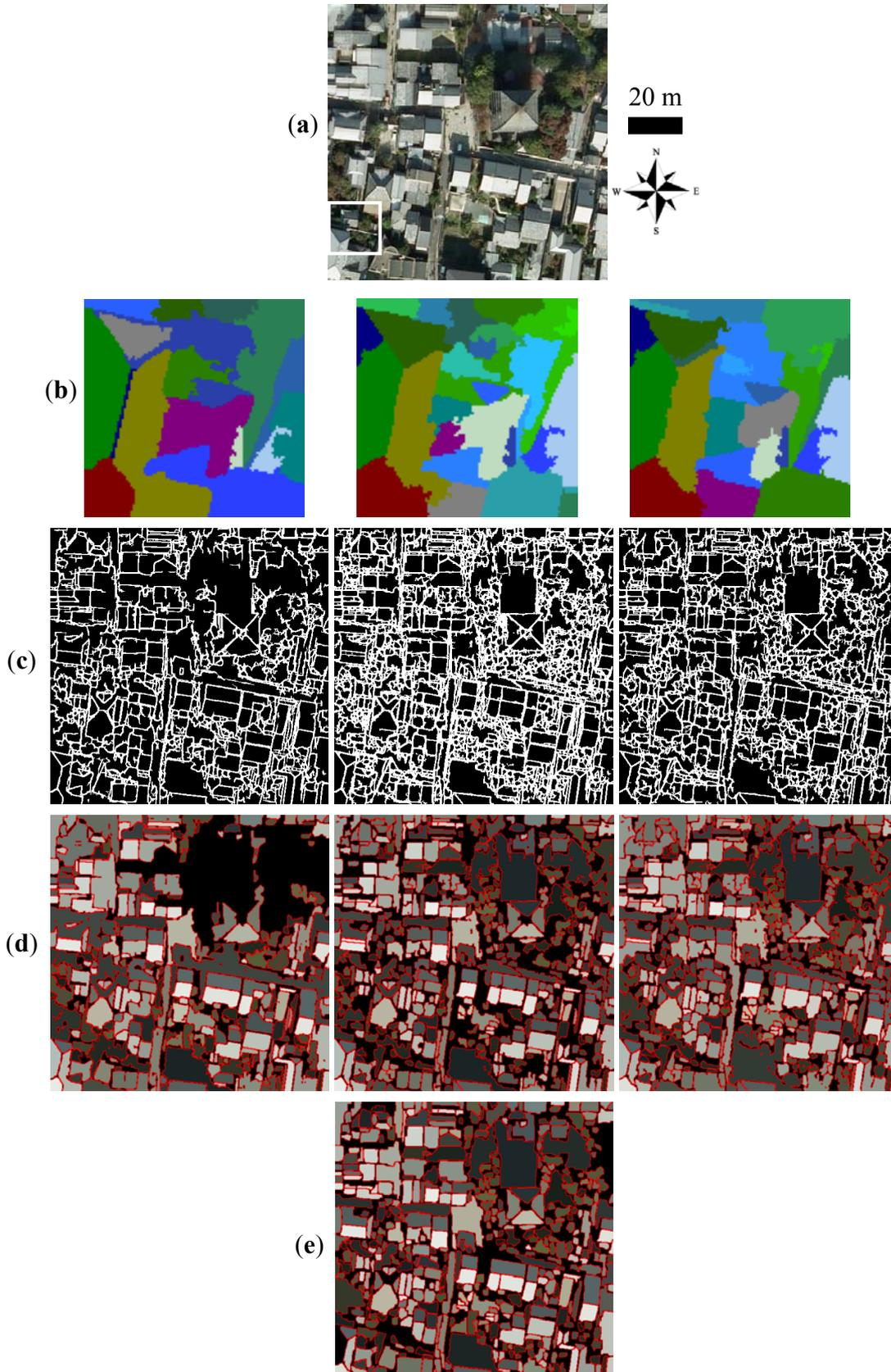
**Figure 6.** Comparison of building segmentation results in Study Area 1, in which low-rise buildings are predominant: (upper) aerial photograph, (lower left) segmentation result using the proposed algorithm, and (lower row) segmentation results using ENVI EX. Parameter values of “Scale Level” and “Merge Level” in ENVI EX were set to 50 and 80, respectively.
