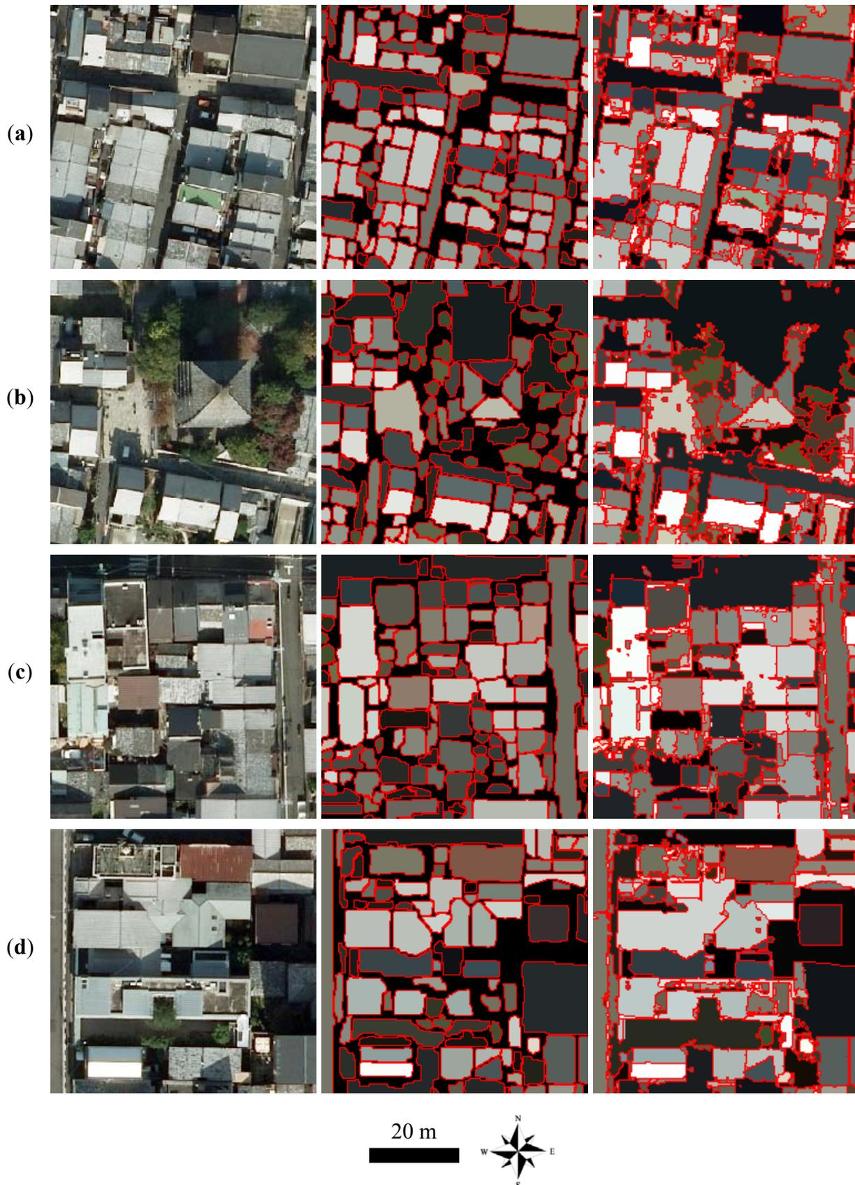
**Figure 14.** Edge completion using filters: (a) non-completed edges, (b) segmentation result using non-completed edges, (c) completed edges, and (d) segmentation result using completed edges. All results were generated with  $\Delta d_i = 40$ .
