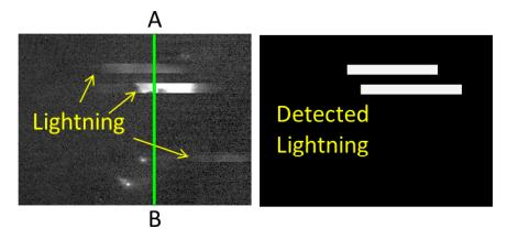
**Figure 10.** Illumination detected from lightning forms horizontal ribbons exactly 16 lines wide, corresponding to the number of lines collected in a single sensor scan. The sample images shows three lightning features. The A-B lines shows the position of the along-track transect presented in Figure 11. The algorithm detected two of the three lightning features.
