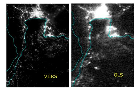
**Figure 1.** Visible Infrared Imaging Radiometer Suite (VIIRS) vs. Operational Linescan System (OLS) low light imaging data collected over Bangkok and the Gulf of Thailand region approximately five hours apart on the night of 14 October 2012. Note that the higher spatial resolution of the VIIRS data enables the detection of a vastly larger number of individual lighting features offshore.
