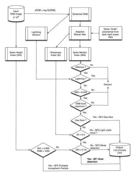
**Figure 2.** Processing flow chart for VIIRS boat detection under low lunar illuminance conditions. The system detects and then assigns them to one of five categories using a quality flag. The highest quality detections are assigned to QF1. QF2 = weaker detections, QF3 = blurry detections, QF4 = gas flares, and QF5 = energetic particle detections.
