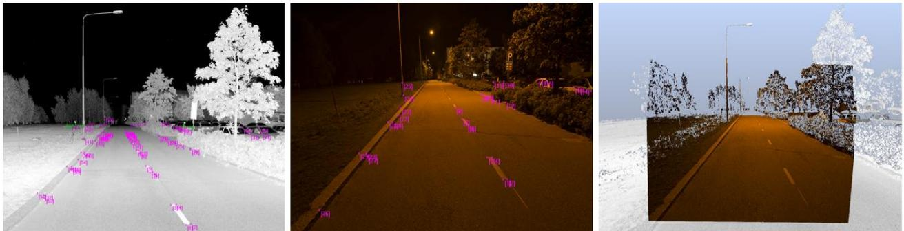
**Figure 4.** Road features such as paintings and kerbstones were used as corresponding points between a TLS-based intensity image and an RGB image for resolving the relative orientation.
