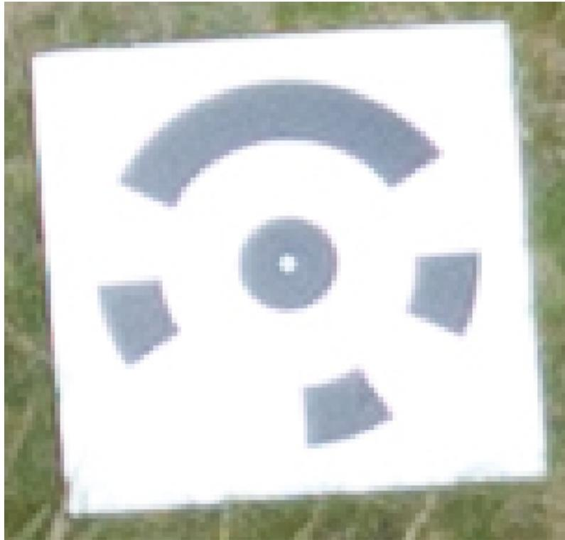
**Figure 2.** A printed PhotoScan coded target as imaged in one of the UAV photographs from the nadir image set.
