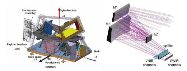
**Figure 1.** Multi-Spectral Instrument (MSI) internal configuration. **Left**: full instrument view (diffuser panel in yellow, telescope mirrors in dark blue). **Right**: optical path construction to the Short-Wave Infrared (SWIR)/visible to near-infrared (VNIR) (see Section 2.2) splitter and focal planes.
