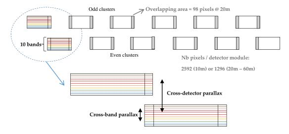
Figure 3. Staggered Detector Configuration.
