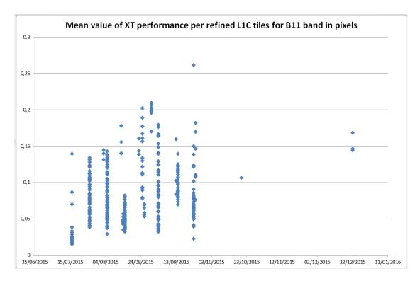
**Figure 55.** Multi-temporal (XT) registration uncertainty for B11 band. Each point represents the average shift measured in one secondary tile with respect to the reference tile.
