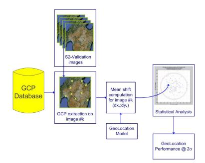
**Figure 43.** General principle of geolocation uncertainty validation using ground control points. Mean shift computation is obtained by correlation technique.
