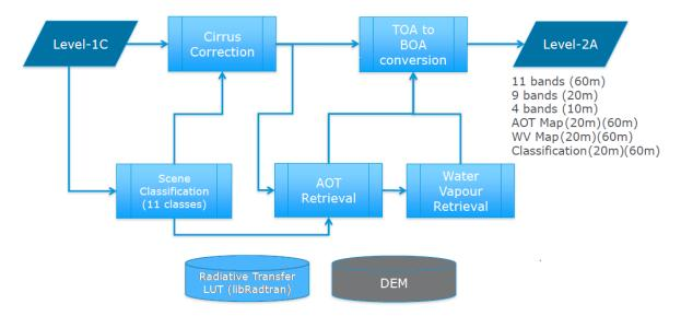
Figure 9. Level-2A processing chain overview.
