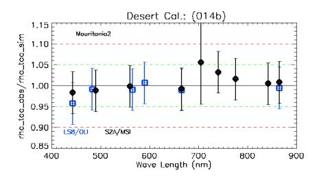
**Figure 37.** Ratio of observed TOA reflectance to simulated one for each sensor (black) S2A/MSI and (blue) LANDSAT-8/Operational Land Imager (OLI) over Algeria3, Libya1, Libya4, and Mauritania2 sites as a function of wavelength. The green (resp. red) dashed lines represent the 5% (resp. 10%) threshold specification. Error bars indicate the estimated uncertainty for the PICS method.
