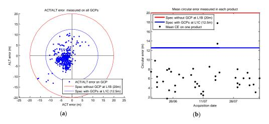
**Figure 46.** System Geolocation Performances in metres for L1C non-refined products. Reference band is B04. (a) Geolocation error (in metre) along-track and across-track measured on each GCP; (b) Mean geolocation error in each product processed in function of the acquisition dates of the product. The two outliers seen on both figures correspond to products from orbit 5601 and are due to contingencies (star-tracker outage).
