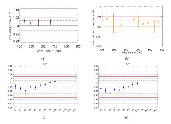
**Figure 28.** Calibration results over (**a**) Rayleigh Scattering; (**b**) ground-based measurements; (**c**,**d**) Deep Convective Clouds. The dashed (resp. solid) red lines represent the 3% goal specification (resp. 5% threshold specification). The reference band is B04 and B07 for (**c**,**d**) respectively. Error bars indicate the estimated uncertainty for Rayleigh and ground-based measurements and the standard deviation for the DCC method.
