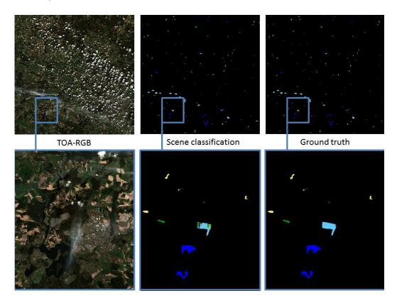
**Figure 62.** Example images for Cloud Screening and Classification Validation analysis, Site Potsdam (Germany), acquired on April 22, 2016, characterized by temperate climate zone and flat terrain. Whole granule at the top and zoomed area at the bottom.
