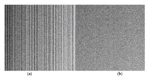
**Figure 24.** Illustration of image equalisation impact: (**a**) Non-equalised diffuser image; (**b**) Equalised diffuser image.
