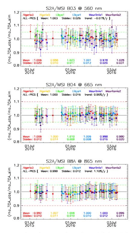
**Figure 32.** Time series of TOA reflectance ratio  $R_b$  from S2A/MSI over (red) Algeria3, (yellow) Algeria5, (green) Libya1, (light-blue) Lybia4, (dark-blue) Mauritania1 and (purple) Mauritania2 for (from top to bottom) B01, B03, B04 and B8A over the commissioning period. The green (resp. red) dashed lines represent the 5% (resp. 10%) threshold specification. Error bars indicate the estimated uncertainty for the pseudo-invariant calibration sites (PICS) method.
