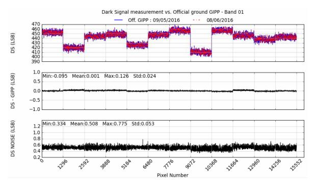
**Figure 10.** Variation of the dark signal measured on 8 June 2016, for the B01 band, with respect to the coefficients calculated from dark acquisition on 9 May 2016. The first plot shows the dark signal level (in digital counts, LSB) as a function of the pixel number, the second plot shows its variation between the two dates, the third plot shows its noise (in LSB).
