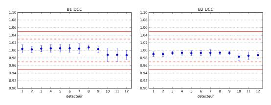
**Figure 30.** B01 (**left**) and B02 (**right**) inter-band calibration coefficients with respect to B04 as a reference band as a function of the detector number, based on Sentinel-2 images calibrated using the diffuser.
