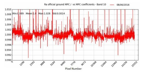
**Figure 13.** R<sub>a</sub> factor as a function of the pixel number (over the 12 detectors) for the update of gain functions measured on 8 June 2016, for the B10 band, with respect to the previous operational coefficients calculated from the sun-diffuser acquisition on 9 May 2016.
