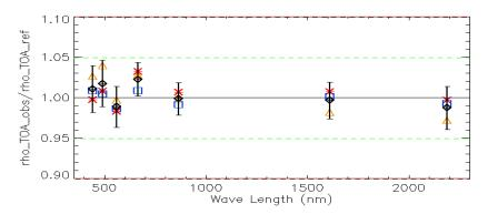
**Figure 35.** TOA reflectance ratio defined as S2A-MSI/LS8-OLI measurements derived from extracted doublets over (red asterisk) Algeria3, (orange triangle) Libya4, (blue square) Railroad Valley Playa site (RRVP) and (black diamond) the average over the three test sites as a function of the wavelength. The green (resp. red) dashed lines represent the 5% (resp. 10%) threshold specification. Error bars indicate the estimated uncertainty.
