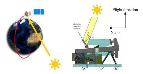
Figure 7. Illustration of the sun diffuser acquisition principle.
