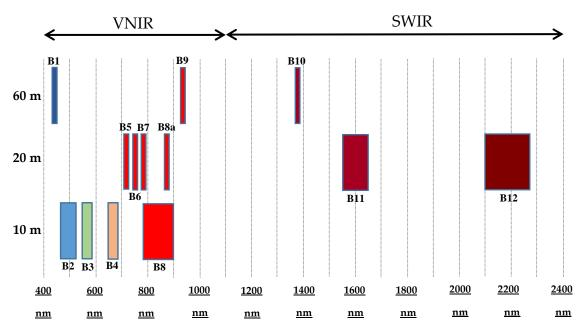
**Figure 2.** MSI spectral bands vs. spatial resolution with corresponding Full Width at Half Maximum (FWHM).
