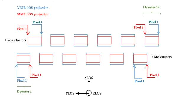
Figure 5. Representation of the pixels Line-Of-Sight (LOS) projection on ground.
