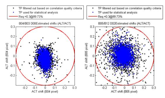
**Figure 49.** Example of global mis-registration shifts measured on 'Central Australia' for B04/B03-Detector 08 and B05/B12-Detector 02. Black points are tie points rejected based on correlation quality criteria (step 4). Units are pixels of the coarser band in the couple.
