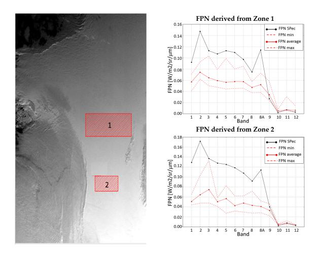
**Figure 26. Left**: Sentinel-2 Greenland image from 2015/09/04 together with the 2 uniform zones that are used to estimate the equalization quality. **Right**: FPN derived independently from the 2 zones.
