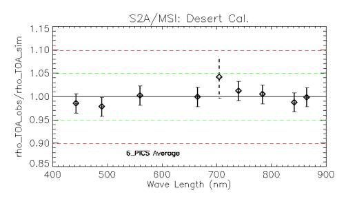
**Figure 33.** Temporal average of the ratio of observed TOA reflectance to simulated one from S2A/MSI over the four-PICS as a function of wavelength. B05 result is shown with black dashed line due to significant gaseous absorption. The green (resp. red) dashed lines represent the 5% (resp. 10%) threshold specification. Error bars indicate the estimated uncertainty for the PICS method.
