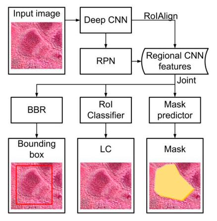
Figure 4. A simplified schematic showing the implementation architecture of the Mask R-CNN.
