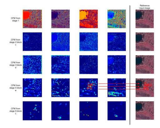
**Figure 13.** Four selected convolutional feature maps (CFM) from the last output layer of the Mask R-CNN stage 1 to 5 for HCPs. Each feature map includes learned features detected across the image. The third CFM in the 4th row provides the geospatial location features for HCPs.
