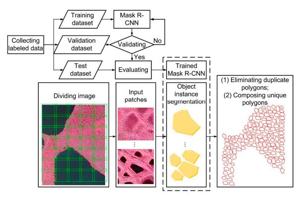
Figure 3. General workflow of automated detection, delineation and classification of ice-wedge polygons.
