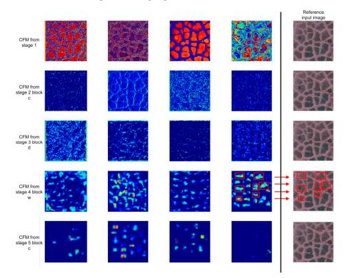
**Figure 14.** Four selected convolutional feature maps (CFM) from the last output layer of the Mask R-CNN stage 1 to 5 for LCPs. Each feature map includes learned features detected across the image. The fourth CFM in the 4th row provides the geospatial location features for LCPs.
