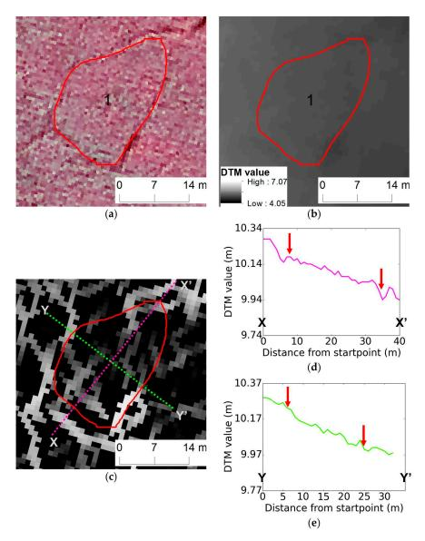
**Figure 17.** Qualitative assessments of incomplete/disjoint IWP extent derived from automated optical imagery mapping (red lines and arrows) to LiDAR data. (**a**) False color composite of VHSR image in 1 m resolution; (**b**) LiDAR-derived DTM at 1 m resolution; (**c**) Canny edge raster from LiDAR DTM; terrain profile of XX" (**d**) and YY' (**e**). The number "1" inside each polygon represent an automated classification as a LCP.
