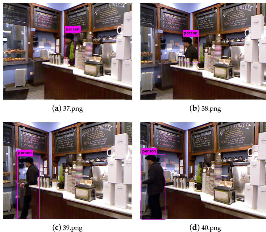
Figure 11. Object detection result of YOLOv3 network.
