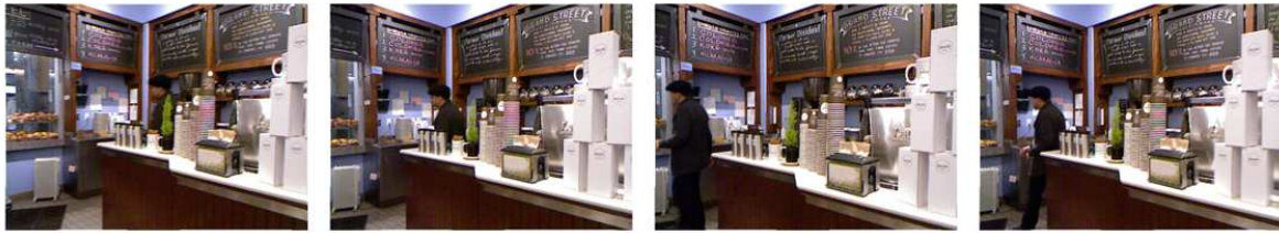
Figure 1. Several keyframe images selected by the traditional visual SLAM system are almost the same, which brings redundant information when constructing maps and reduces the efficiency of mapping.
