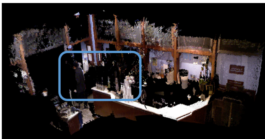
Figure 10. Dense point cloud map constructed by our method.
