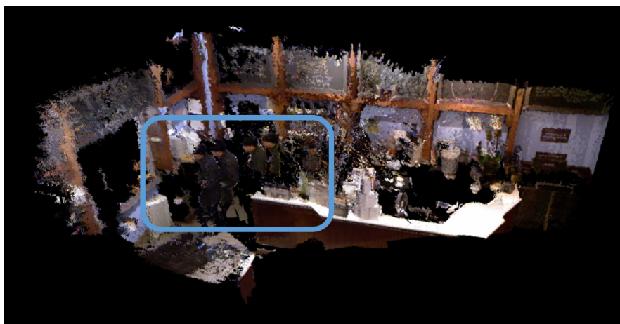
Figure 2. Dense point cloud map constructed by keyframe-based SLAM. We can find that pedestrians in the scene also appear in the map, which will bring many difficulties to the application of the map, such as path planning.
