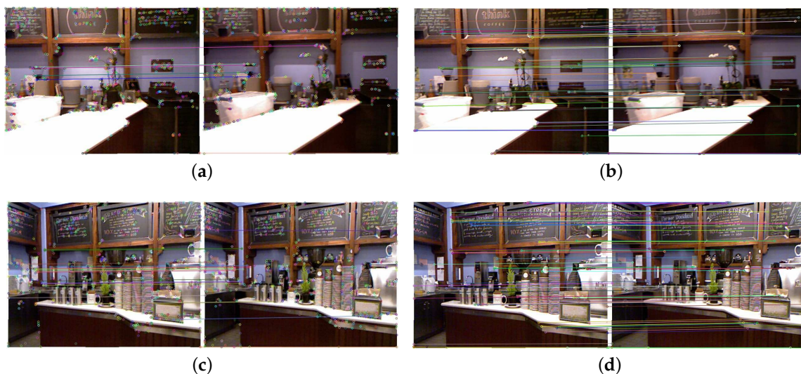
Figure 7. (a,c) extract feature points in the whole image, (b,d) divide the image equally into 16 cells and extract feature points in every cell. We find that the feature points in (b,d) are significantly more than (a,c), and the feature points are more evenly distributed. (a) Extract feature points in whole image, and good match condition is 5 times the minimum distance. (b) Divide image equally into 16 cells and extract feature points. (c) Extract feature points in whole image, and good match condition is 5 times the minimum distance. (d) Divide image equally into 16 cells and extract feature points.
