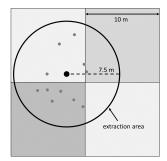
**Figure 4.** Exemplary extraction area of 176.7 m<sup>2</sup> with 10 m pixels in the background. The center of the circle represents the centroid of the sampling locations of all dates (grey dots).
