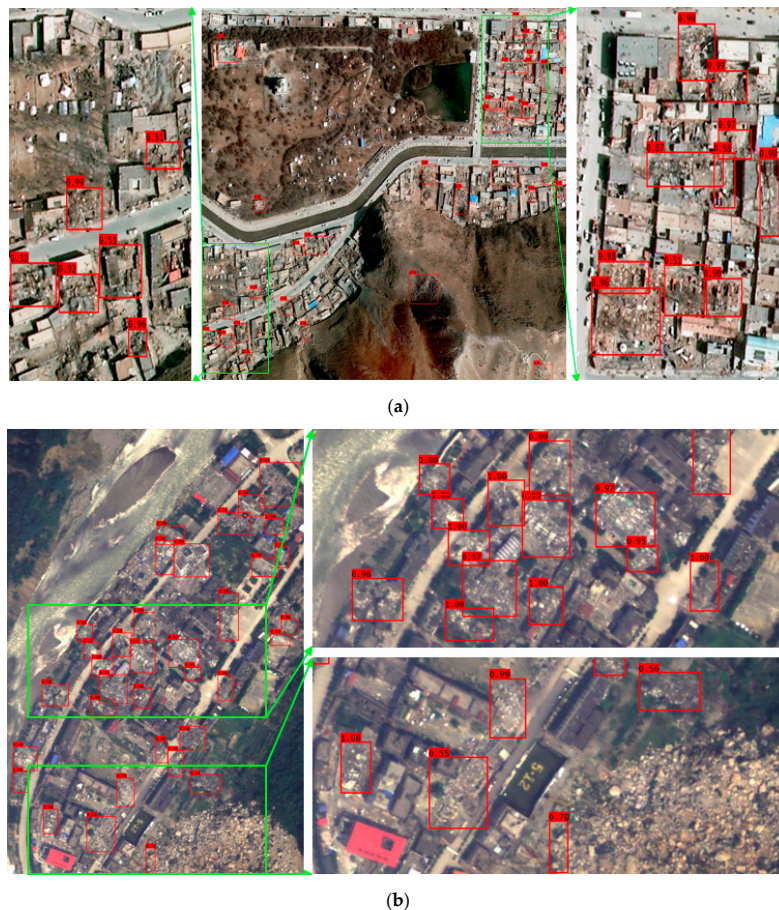
Figure 17. Example of YOLOv3-S-GIoU model detection results. (a) Test image for the Yushu earthquake; (b) test image for the Wenchuan earthquake
