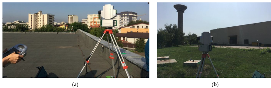
Figure 6. TLS point clouds acquisition using the Maptek I-Site 8820 terrestrial laser scanner, from station point C (a) and A (b).
