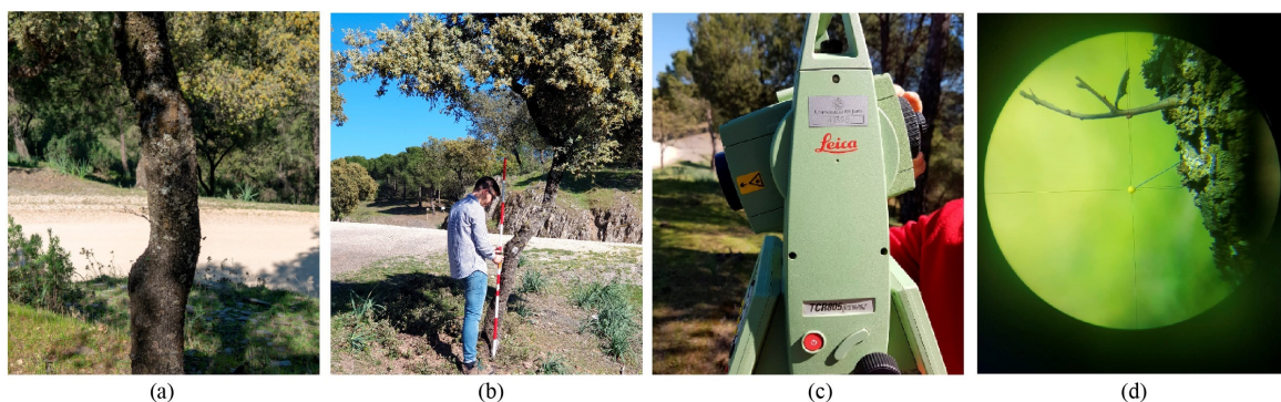
Figure 8. Field measurements of structural parameters of trees. (a) The target tree, (b) The manually marking of the lowest point of the tree trunk, (c) Leica TCR-805 (TS); and (d) The view of the pointing to the pin on each side of the trunk.
