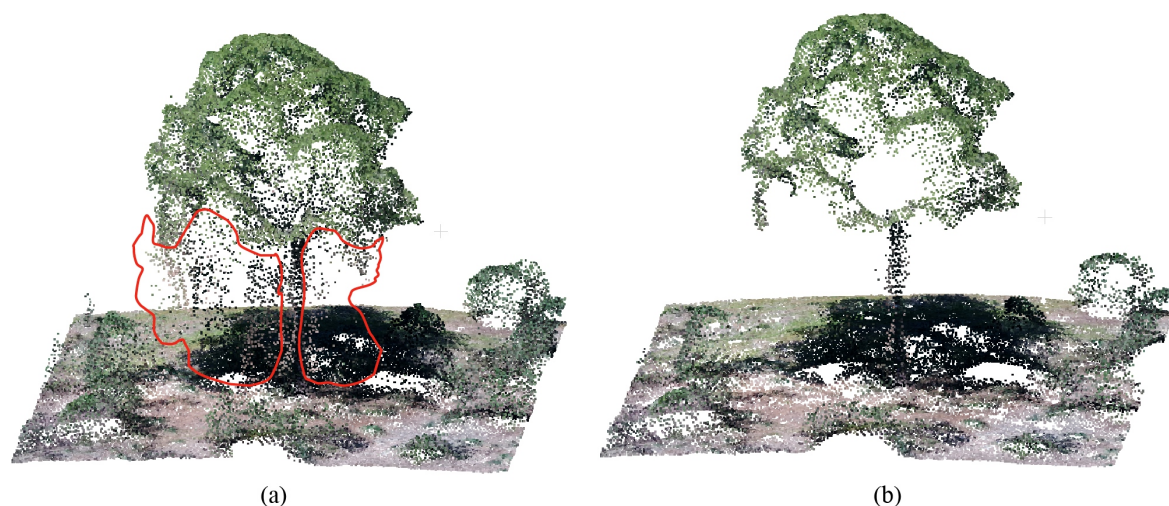
Figure 4. The point-based filter of a cutout of the point cloud. (a) The original dense point cloud; and (b) The filtered point cloud.
