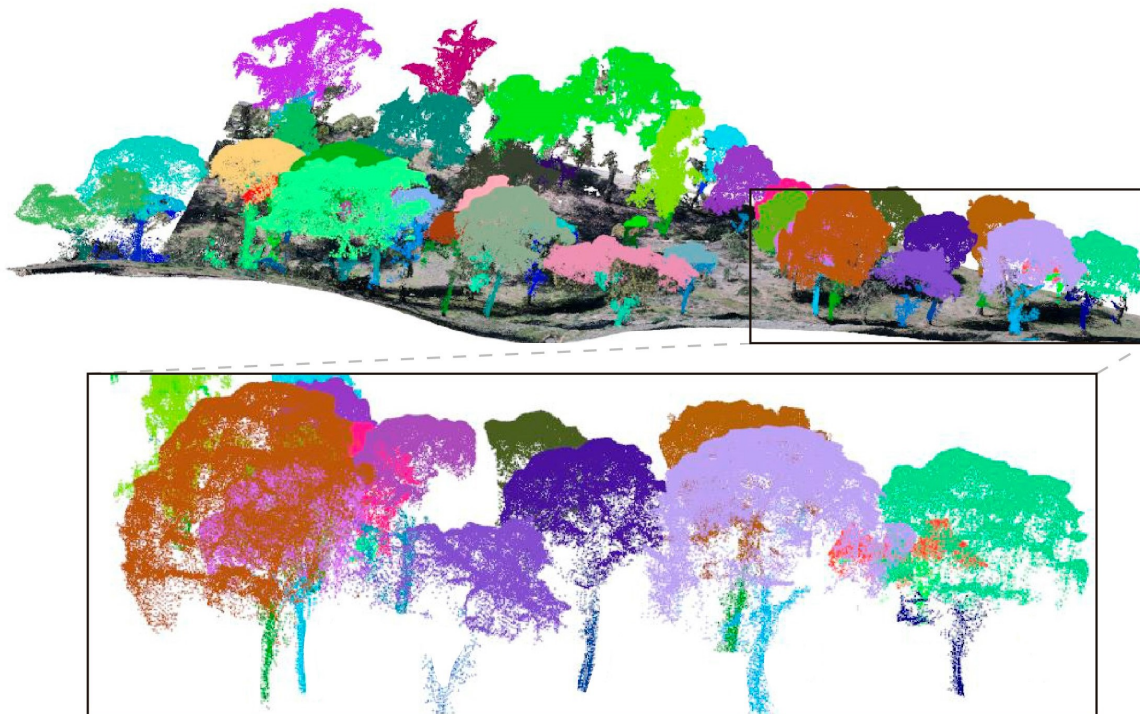
Figure 10. The segmentation of individual trees and the recognition of the crown and trunk for each tree.
