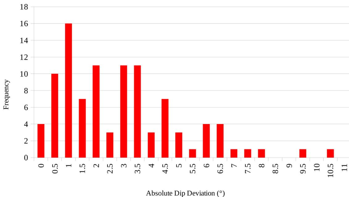
**Figure 15.** Histogram of pre-split holes' absolute dip deviation for Mine C assessed using the UAV photogrammetric model shown in Figure 14. A total of 100 pre-split hole measurements are included in this histogram.
