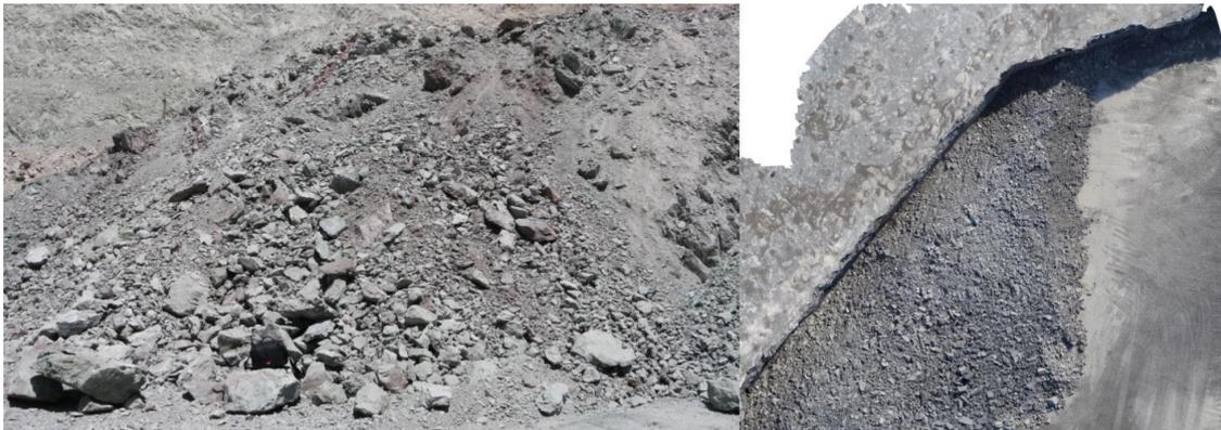
**Figure 9.** Images from Mine A (left) and Mine B (right) produced for image analysis of the blasted muck piles.
