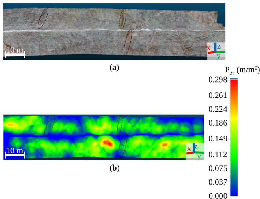
**Figure 3.** (a) Section of Mine D pit mapped (two benches). (b)  $P_{21}$  fracture intensity mapped on the pit wall (red represents higher fracture intensity zones, and blue represent lower fracture intensity areas).
