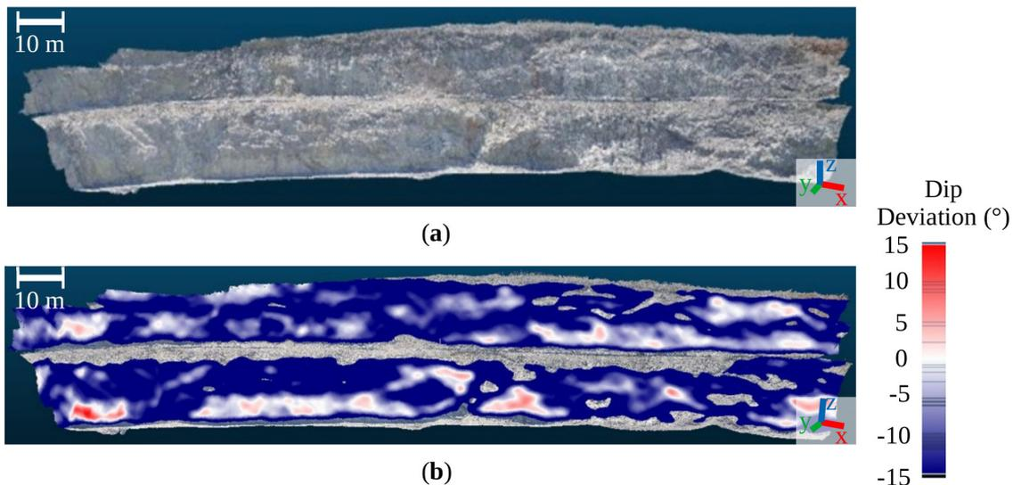
**Figure 13.** (a) Point cloud generated for Mine A and (b) the achieved bench face angle compared to the target bench face angle of  $75^\circ$ , with areas in blue lower, white  $\pm 3^\circ$  of the target and red as areas above the target.
