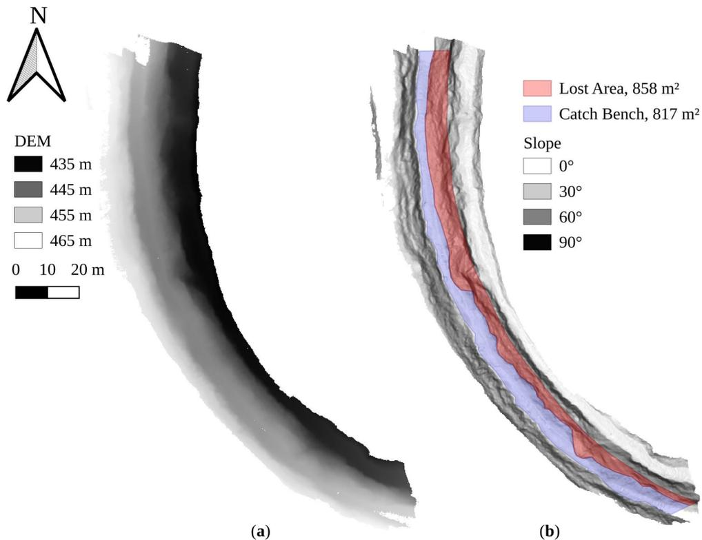
**Figure 11.** (a) DEM of Mine A. (b) Raster representing the slope used for bench width analysis. The actual catch bench area is shown in light blue, and the blast-induced overbreak causing lost area is shown in light red.
