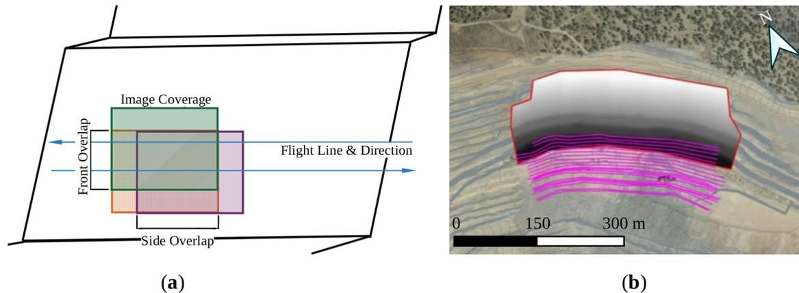
**Figure 1.** (a) Schematic of the overlap and flight path design for pit wall mapping. (b) Flight plan design for Mine D; the flight paths are shown in magenta, and the area of interest is outlined in red with the DEM inside the outline.
