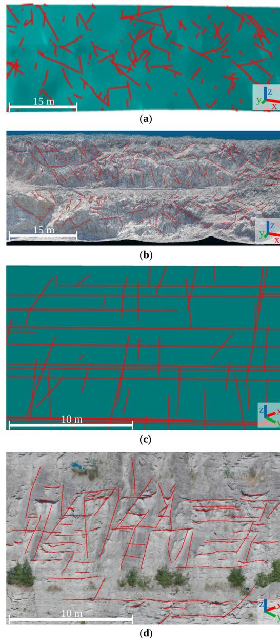
**Figure 4.** Trace-planes of DFN models (green) generated for (a) Mine A and (c) Mine B. Red lines represent joint traces. Trace-planes of UAV virtual mapping generated for (b) Mine A and (d) Mine B.
