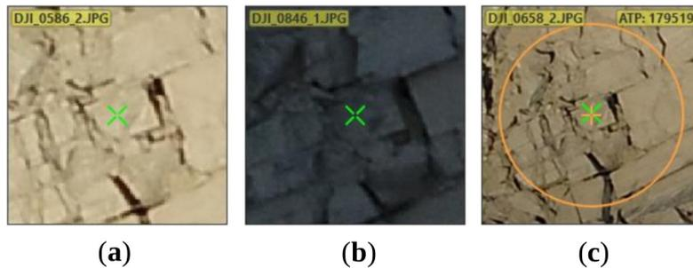
**Figure 19.** Images captured during a single flight using the same lens, filter, focal length and camera settings. The same location on the pit wall is identified by the green cross. (a) High glare caused by direct sunlight, (b) fully shaded and (c) indirect lighting environments were encountered while a shadow moved up the pit wall.
