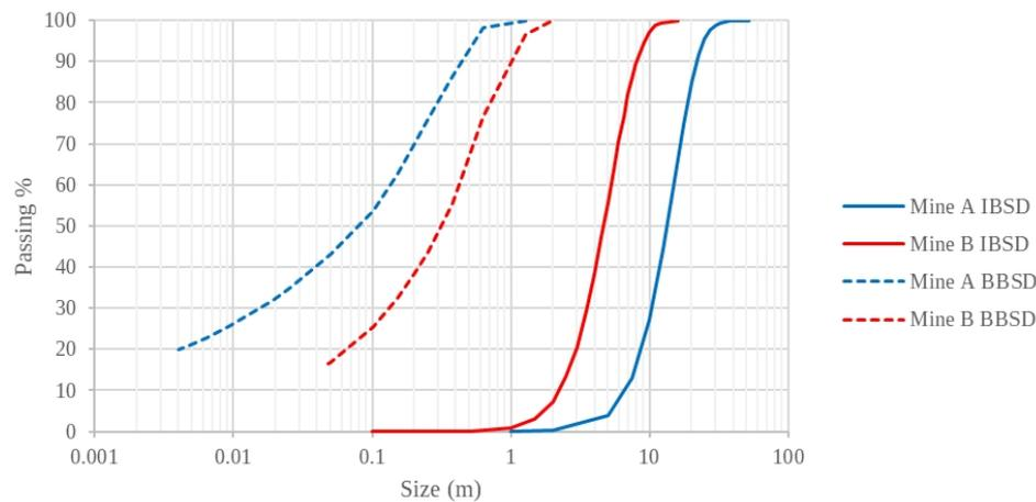
**Figure 6.** Particle size distribution plots for Mines A and B. The IBSDs estimated using DFN models are illustrated with solid lines. The BBSDs measured using image analysis for Mines A and B are drawn using dashed lines. BBSD measurement is described in Section 5.1.
