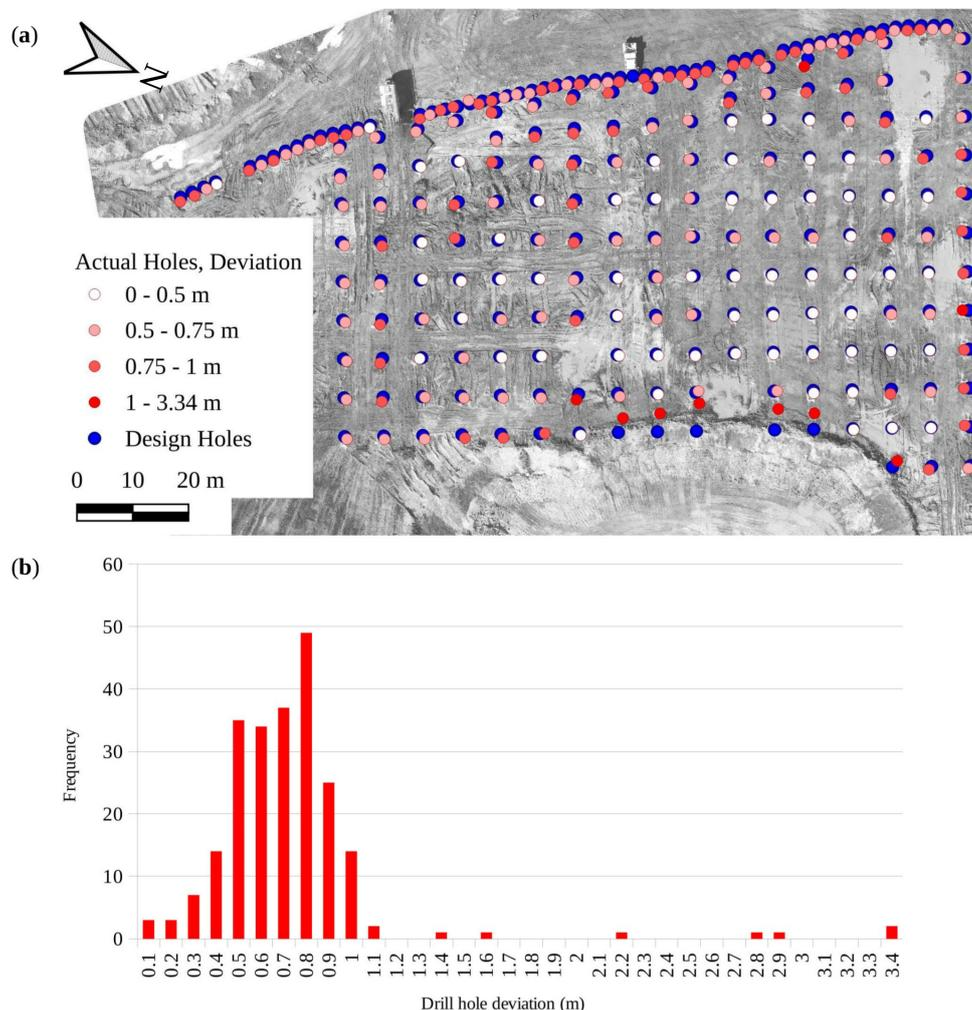
**Figure 7.** Blasthole deviation analysis for 230 holes with a diameter of 225 mm at the blast location in Mine D. (a) Orthomosaic with the designed (blue) and implemented (gradient red) blast pattern. (b) Histogram of visible drill hole collar deviation for the implemented blast pattern.
