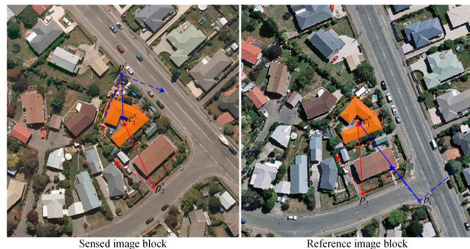
Figure 8. Illustration of the cross-validation. p_1^s and p_1^r are a pair of matching key points given by SIFT, as well as p_2^s and p_2^r . The dashed arrow indicates the SIFT major orientation of each key point, that is, the positive direction of the x-axis of its coordinate system. Each dashed line without an arrow indicates the positive direction of the y-axis (note that the original positive direction of the y-axis in the image coordinate system is downward). c_1^s and c_1^r denote the centers of the minimum enclosing circles of the center instances. The solid arrow indicates the relative position vector of each key point. In this example, \vec{p_1^s c_1^s} is (46.965, 110.409), and \vec{p_1^r c_1^r} is (260.657, 9.204). Their Euclidean distance is 236.446. \vec{p_2^s c_1^s} is (158.180, 99.205), and \vec{p_2^r c_1^r} is (160.201, 96.003). Their Euclidean distance is 3.787. Therefore, p_1^s and p_1^r are key points of mismatch and eliminated. The process only involves a basic analytical geometry method, so we do not elaborate on it here.
