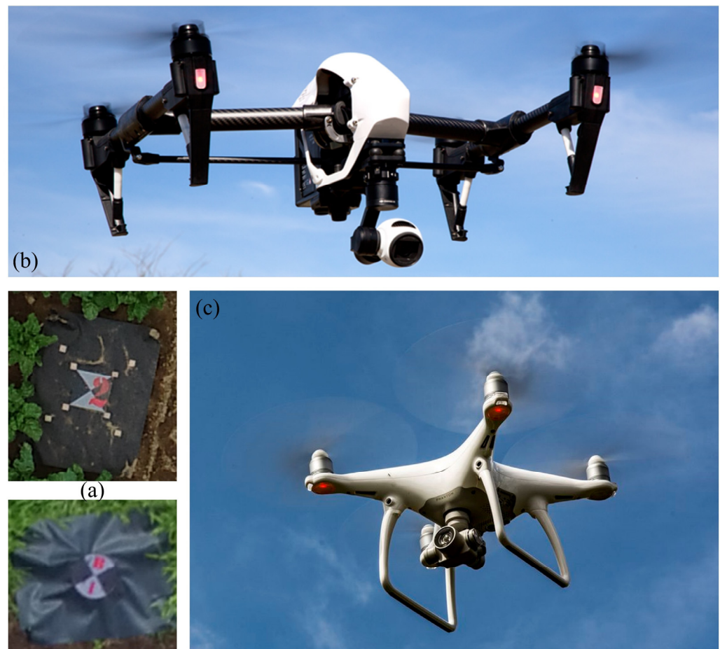
Figure A2. Ground control point (GCP) and unmanned aerial vehicle (UAV) systems used in the field. (a) Square and circle GCPs, (b) DJI Inspire 1, and (c) DJI Phantom 4 (V1 and V2 share a similar appearance).
