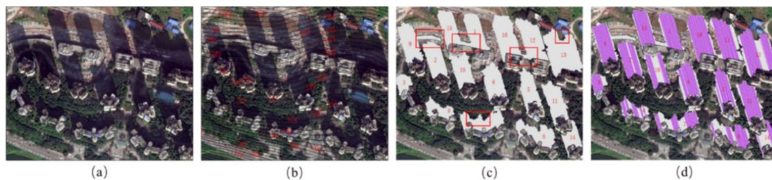
**Figure 16.** Visual display of building height estimation in complex terrain. (a) Original image; (b) Contour lines; (c) Shadow boundary; (d) Final result of shadow lines.
