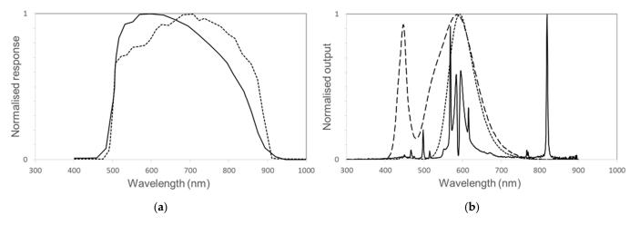
**Figure 1.** Typical normalized spectral response of satellite sensors and selected streetlighting types. (**a**) the DMSP-OLS (solid line) and VIIRS-DNB (dashed line) sensors, compared with (**b**) normalized output of high pressure sodium (solid line), 1800 K LED (short dashes) and 4000 K LED (long dashes) streetlights.
