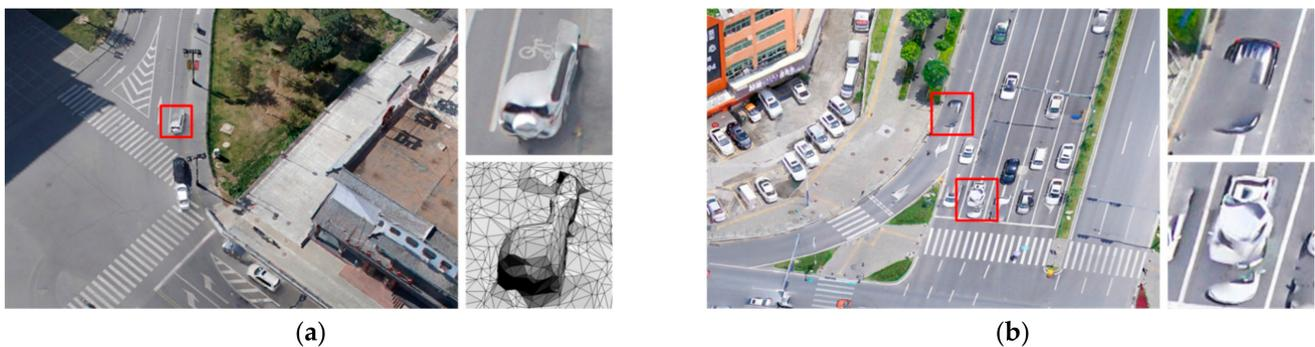
**Figure 1.** The influence of moving cars on the 3D reconstruction results, in which Figure (a) displays the mesh deformation and Figure (b) displays the texture distortion.
