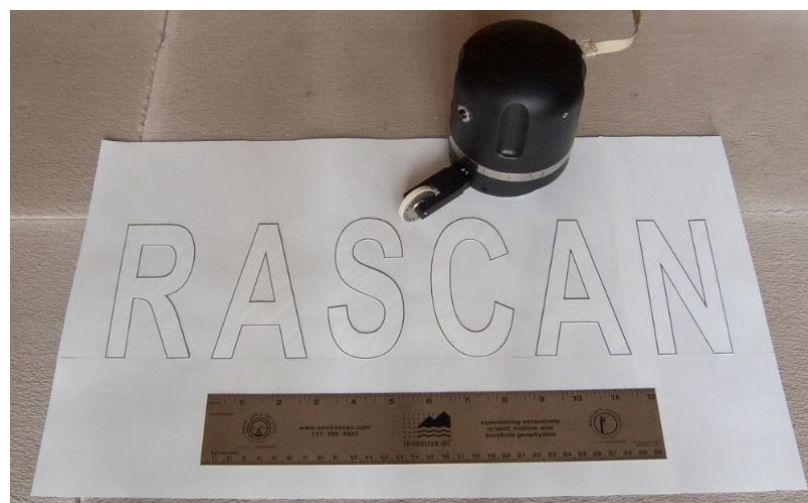
Figure 5. Paper sheet with aluminum foil letters (ruler is 12 inches, or 30.48 cm).
