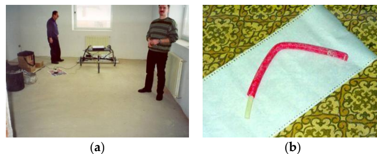
Figure 22. (a) MiRascan radar at work and (b) sample of plastic tubing.
