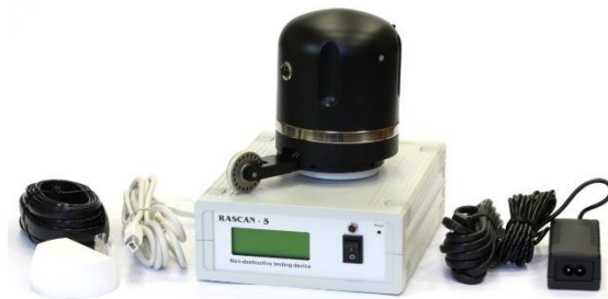
Figure 10. Holographic subsurface radar RASCAN-5 [64].
