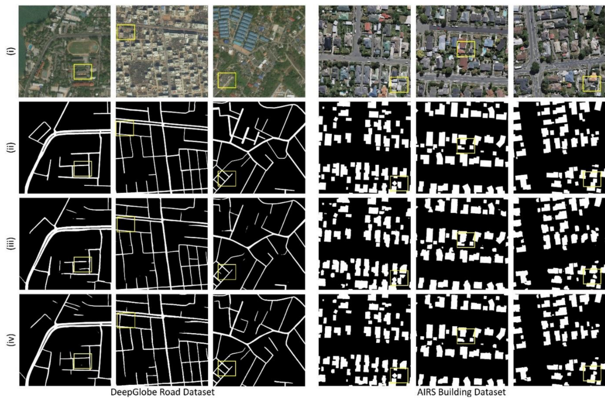
Figure 12. Building and road maps produced by the presented BCL-UNet and MCG-UNet techniques from the AIRS and DeepGlobe datasets. (i) Original imagery, (ii) ground truth imagery, (iii) results of BCL-UNet, and (iv) results of MCG-UNet. The yellow boxes present the predicted FPs and FNs.
