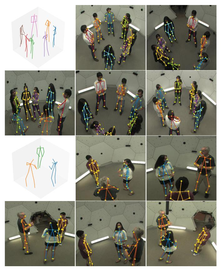
**Figure 7.** Experiment results on two different types of multi-people scenes. The 2D poses in each view are obtained by reprojecting 3D poses to camera coordinates via camera parameters. **Top**: Dense scene with 7 people in total. *MAO-Pose* is able to reconstruct all the peoples using 5 views. **Bottom**: Sparser scene with only 3 people.
