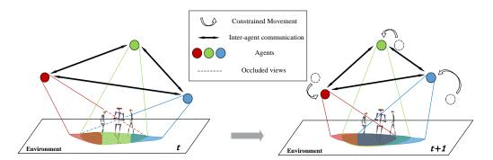
**Figure 1.** Illustration of how agents operate online view selection from time step t to t + 1, here shown for a triple-agent scenario. At time step t, agents observe the environment with multiple views among which some are occluded by human bodies (shown as colored dash lines). To avoid the current occlusion and get a more accurate estimation of human poses, agents jointly move to new viewpoints at the next time step t + 1, which are generated by the learnt policy.
