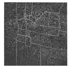
**Figure 5.** Long before GIS, overlay of cadastral boundaries using photographic techniques was trialled and applied, including in Africa (adapted from [75]).
