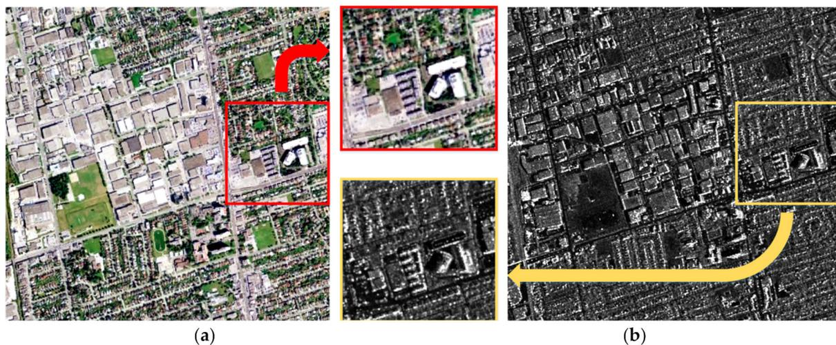
**Figure 4.** An example of radiation difference between MMRS images: (a) Optical image. (b) SAR image. As shown by the enlarged patch, the radiation differences and noise effects are particularly noticeable.
