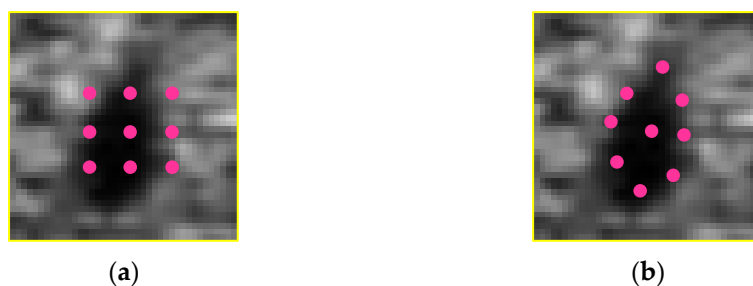
Figure 10. Different convolutions. (a) Classical convolution; (b) deformation convolution.
