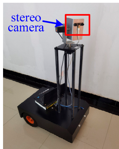
Figure 10. Stereo camera and simulated planetary rover.
