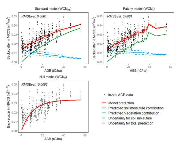
**Figure 5.** In situ AGBC data and fitted forward WCM<sub>s</sub> (WCM<sub>std</sub>, WCM<sub>k</sub>, and WCM<sub>0</sub>) with separate lines illustrating model prediction of total backscatter, vegetation contribution, and soil moisture contribution, covering the range of observed values (0–60 tC/ha). Total backscatter is expressed in normalised radar cross-section (NRCS,  $m^2/m^2$ ). Fitted parameters a, b, c, and d are provided in Table A2.
