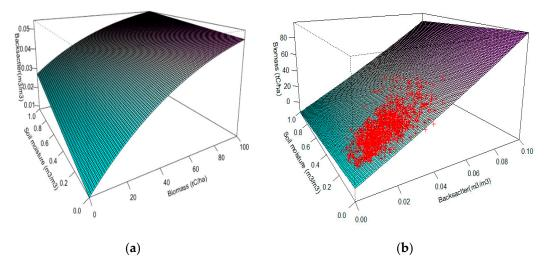
**Figure A2.** Prediction surface from the fitted WCM<sub>std</sub> (**a**) and BM-WCM<sub>std</sub> (**b**) with the calibration data plotted in red points.
