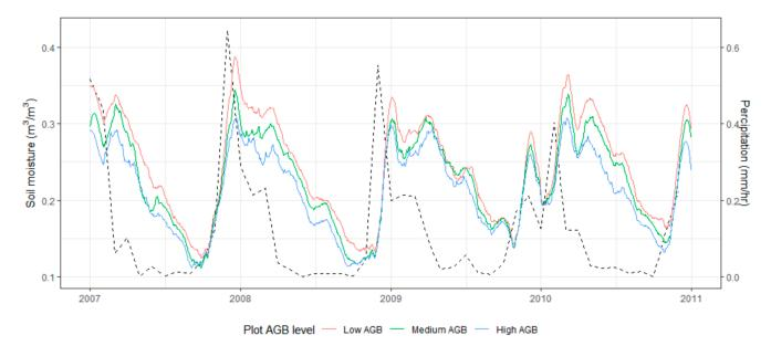
**Figure 3.** Change in soil moisture for three example plots with low (12 tC/ha, red line), medium (23 tC/ha, green line), and high (50 tC/ha, blue line) AGBC. Monthly precipitation estimates (dotted line) were plotted from Tropical Rainfall Measuring Mission (TRMM) data version 3B43 v7 from Google Earth Engine [53]. Note that monthly precipitation estimates are given in mm/h.
