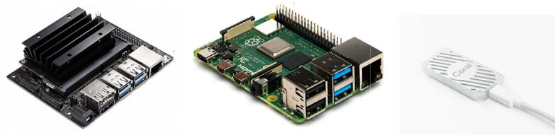
Figure 3. From left to right: Jetson nano, Raspberrypi, and Google TPU Coral.
