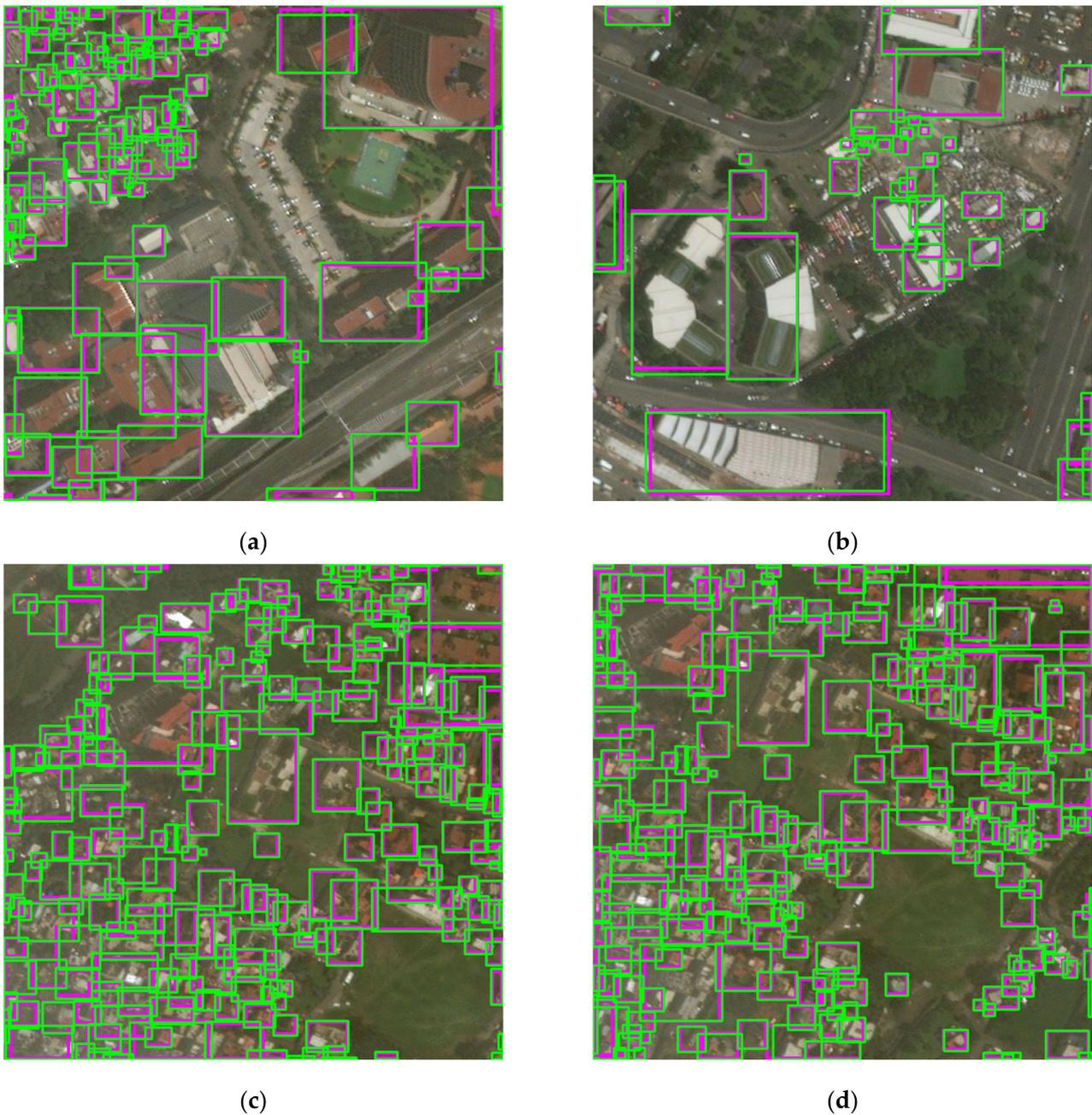
**Figure 10.** Representative test results of small dense post-earthquake buildings (green: ground truth, pink: predicted bounding box): (a) Example 1; (b) Example 2; (c) Example 3; (d) Example 4.
