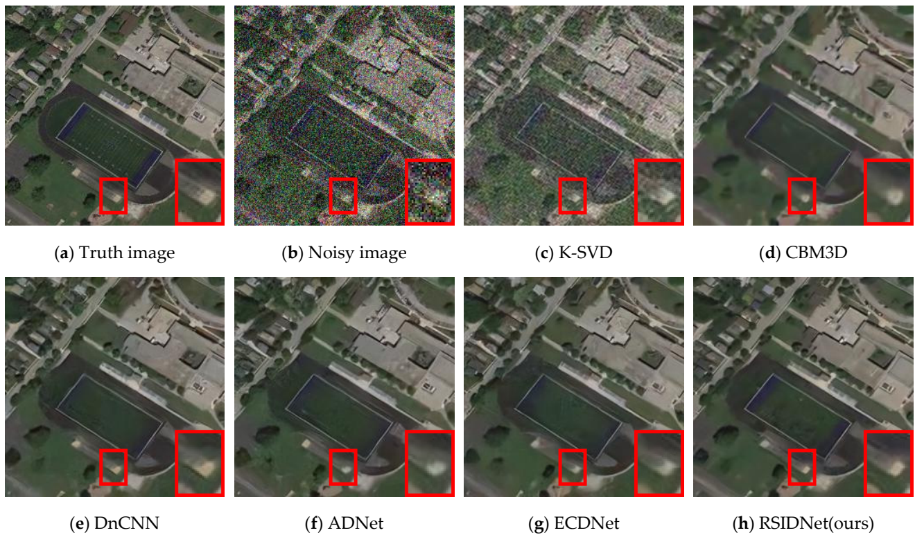
Figure 11. The denoising effects of various methods when the noise intensity is \sigma = 50 . The PSNR values are: (b) noisy image, 14.81 dB; (c) K-SVD, 24.76 dB; (d) BM3D, 27.03 dB; (e) DnCNN, 27.97 dB; (f) ADNet, 27.95 dB; (g) ECNDNet, 27.96 dB; (h) RSIDNet(ours), 28.11 dB.
