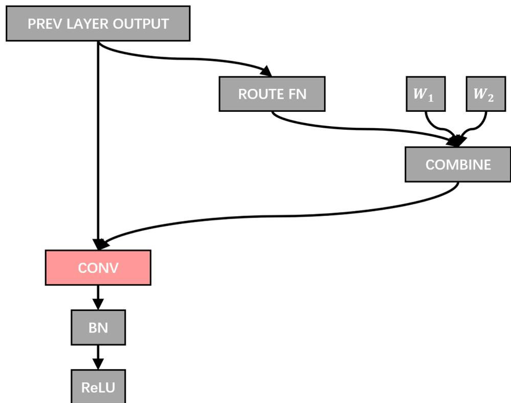
**Figure 6.** CondConv [78] layer architecture with  $n = 2$  kernels. CondConv:  $(\alpha_1 W_1 + \alpha_2 W_2) \times x$ .
