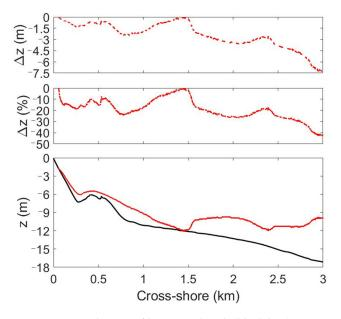
**Figure 5.** Cross-shore profile at Mira beach (black line) versus estimated water depths and respective errors and relative errors using constant  $\lambda_0$  (red line and red dotted line).
