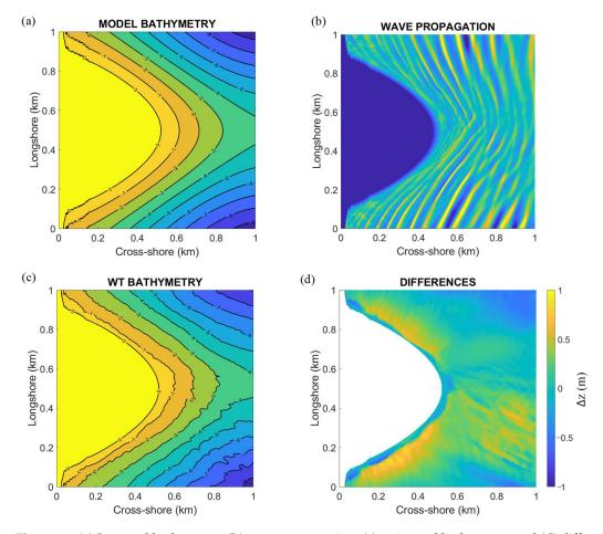
Figure 10. (a) Imposed bathymetry, (b) wave propagation, (c) estimated bathymetry and (d) differences between both bathymetries.
