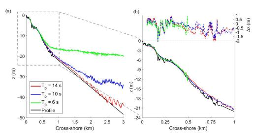
**Figure 8.** (a) Real cross-shore profile at Carvalhido beach (black line) versus estimated water depths using  $T_p = 6$  s (green),  $T_p = 10$  s (blue) and  $T_p = 14$  s (red). (b) Details along the first kilometer show the respective estimation errors.
