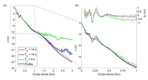
**Figure 9.** (a) Real cross-shore profile at Baleal beach (black line) versus estimated water depths and respective errors using  $T_p = 6$  s (green),  $T_p = 10$  s (blue) and  $T_p = 14$  s (red). (b) Details along the first kilometer and showing the respective estimation errors.
