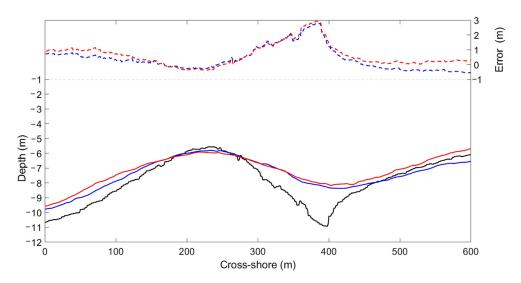
**Figure 13.** Measured bathymetry profile (black line) versus estimated water depths on 1 December 2020 (blue) and on 2 December 2020 (red) and respective errors.
