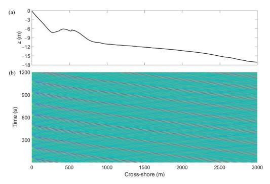
**Figure 4.** (a) Mira Beach cross-shore profile; (b) corresponding timestack, using FUNWAVE numerical simulations performed with  $H_s = 1$  m and  $T_p = 10$  s.
