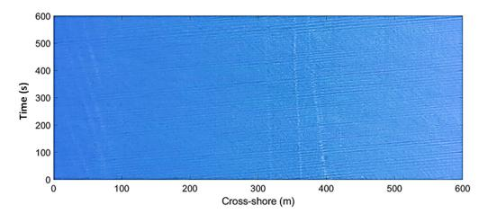
**Figure 12.** Example of the 10-min Timestack generated by the camera on 1 December 2020 (12:50–13:00).
