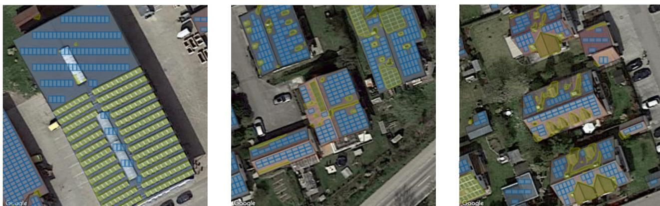
**Figure 11.** Examples of roof segments (light gray), roof superstructures (green), and module placement (blue) in the study area.
