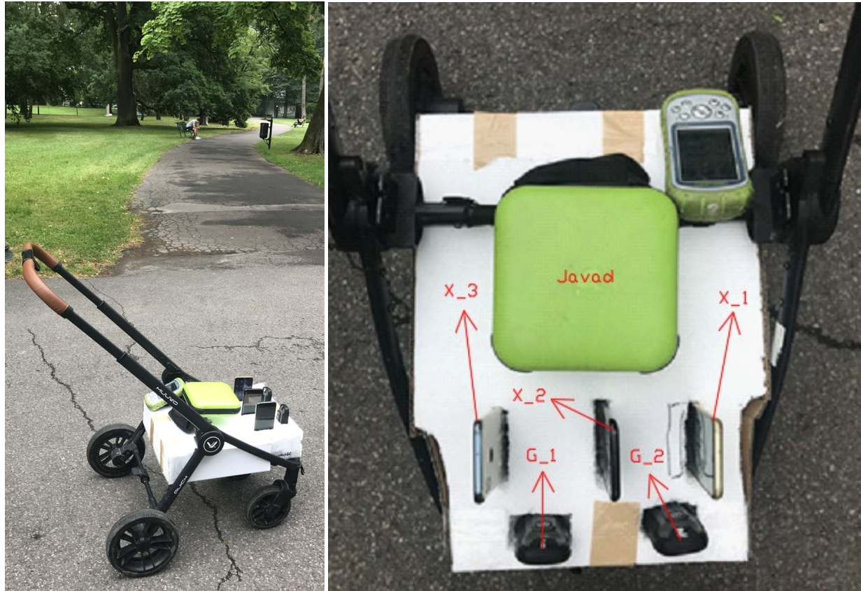
Figure 3. Survey equipment design and GNSS devices used in the study.
