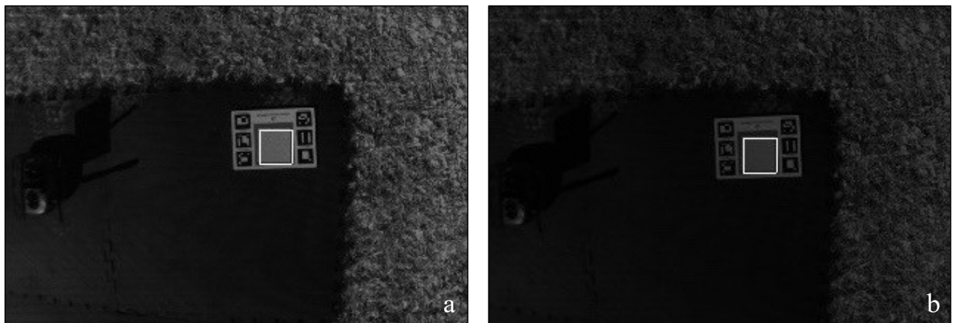
Figure 6. Radiometric calibration plate used to convert raw digital numbers (a) to reflectance values (b).
