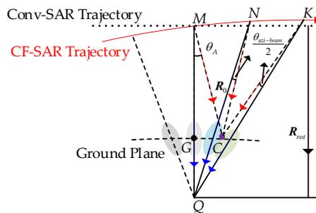
Figure 10. Schematic of the synthetic aperture of CF-SAR.
