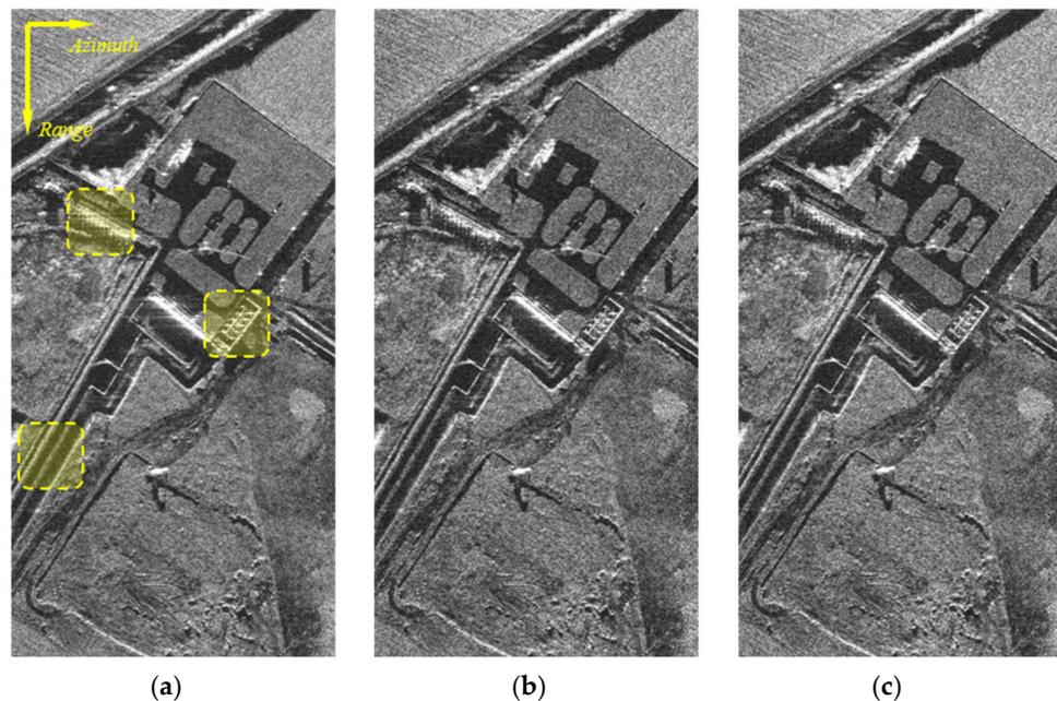
**Figure 13.** Real data experiment results of the high-resolution UAV-borne Ka-band CF-SAR. (a) Result processed by RDA. (b) Result processed by FFBPA. (c) Result processed by the algorithm proposed in [8].
