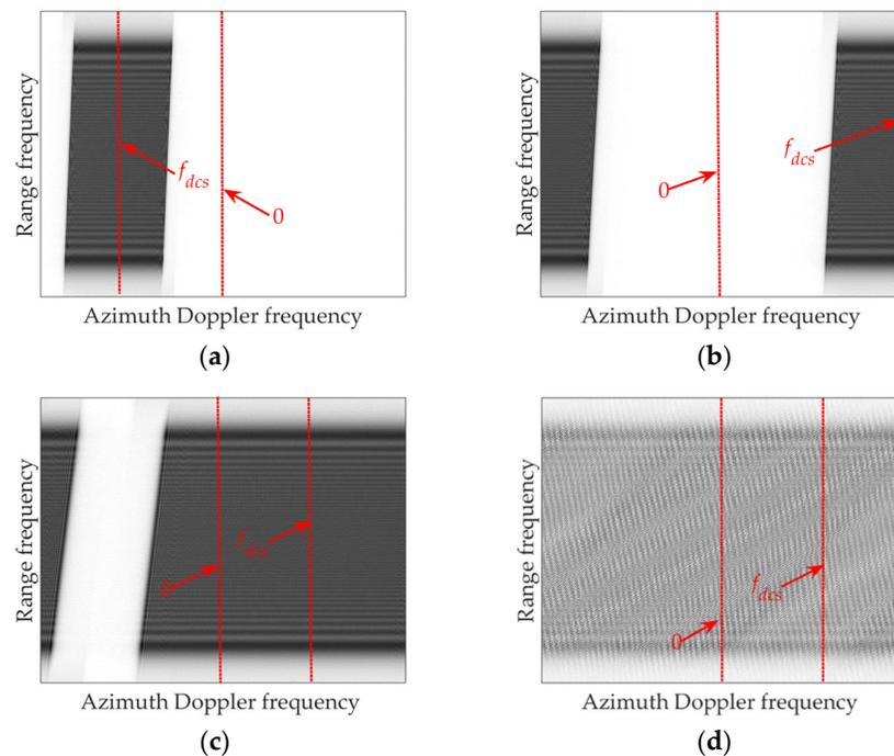
**Figure 14.** Theoretical 2D spectrum distributions of a moving target for CF-SAR: (a) spectrum entirely in a PRF band; (b) spectrum spanning neighboring PRF; (c) Doppler bandwidth exceeding PRF/2; and (d) Doppler bandwidth exceeding the PRF.
