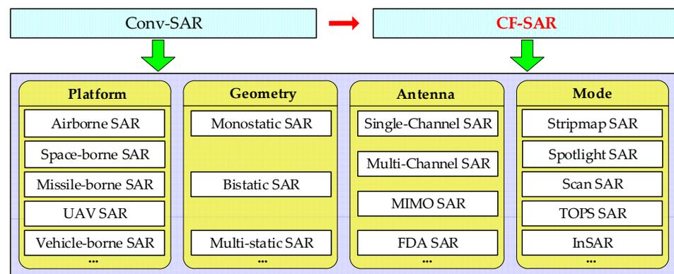
**Figure 2.** Schematic diagram of the classification of CF-SAR. The full names of some acronyms are as follows: UAV is unmanned aerial vehicle, MIMO is multi-input multi output, FDA is frequency diversity array, TOPS is terrain observation by progressive scans, and InSAR is interferometric SAR.
