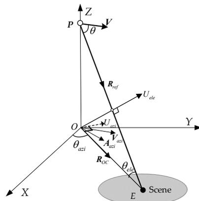
**Figure 9.** Space geometry and mechanics projection mapping relationship of CF-SAR.
