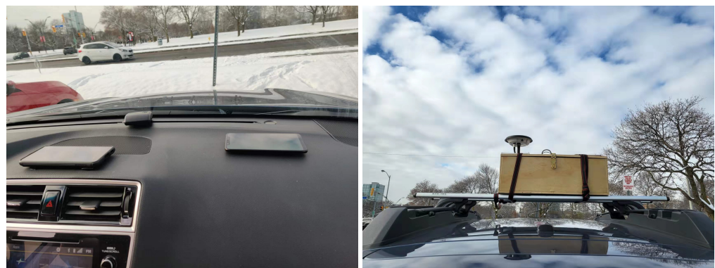
Figure 3. Photos of strapped reference sensors used in measurement campaigns.
