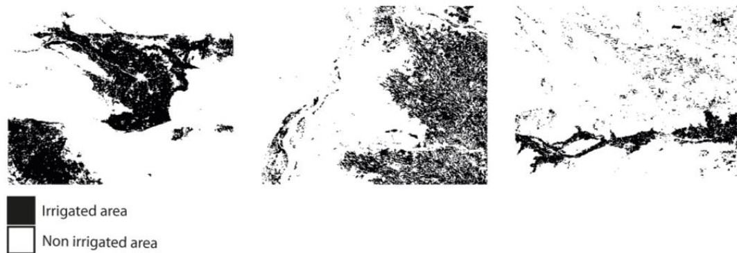
Figure 6. Irrigated area of 2016 derived from PROBA-V data at 10 arc seconds (approx. 300 m) for the regions of China (left), Sudan (middle) and USA (right).
