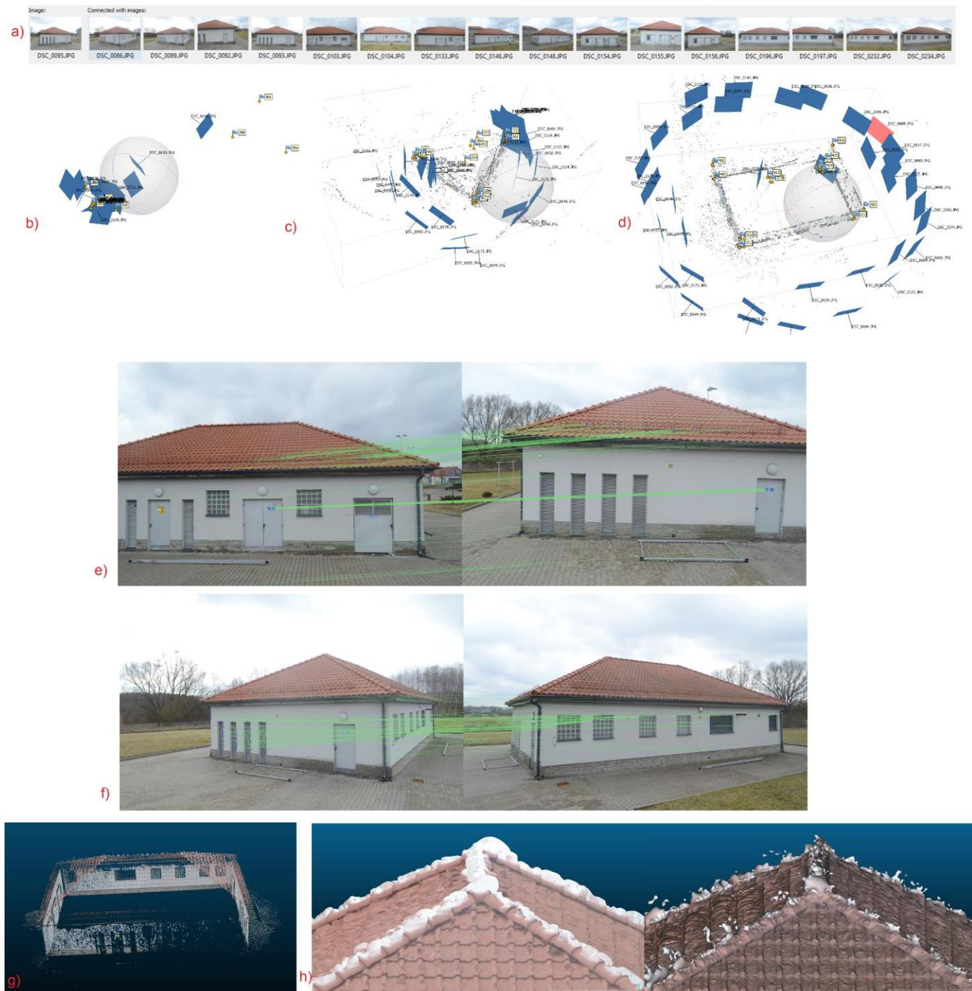
**Figure 15.** Software problems in processing the CRBeDaSet: (a) faulty matching of tie points; (b–d) the examples of the problems with optimal selection of tie points and weight assignment; matching problems related to (e) repeated regular shapes and color of roofing tiles and (f) localization of windows and vent holes near homogenous texture of wall; (g) shortages in point clouds; (h) difficulty with correct automatic filtering of dense point clouds during the mesh generation.
