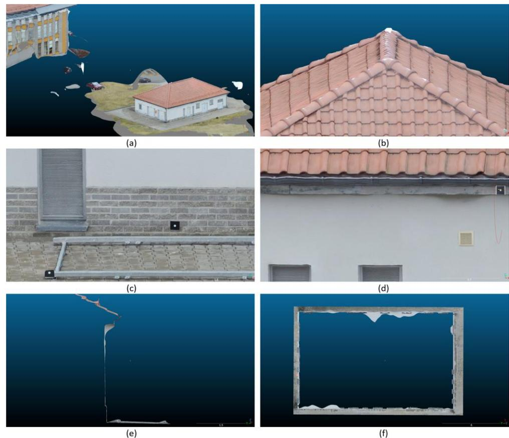
**Figure 10.** ContextCapture 3D mesh model: (a) general look on generated mesh 3D model; (b) roof geometry reconstruction; (c) façade with clinker tiles and wall without visible texture; (d) corners of the building roof and wall without visible texture; (e) vertical section of elevation 1; (f) top view on the building without a roof.
